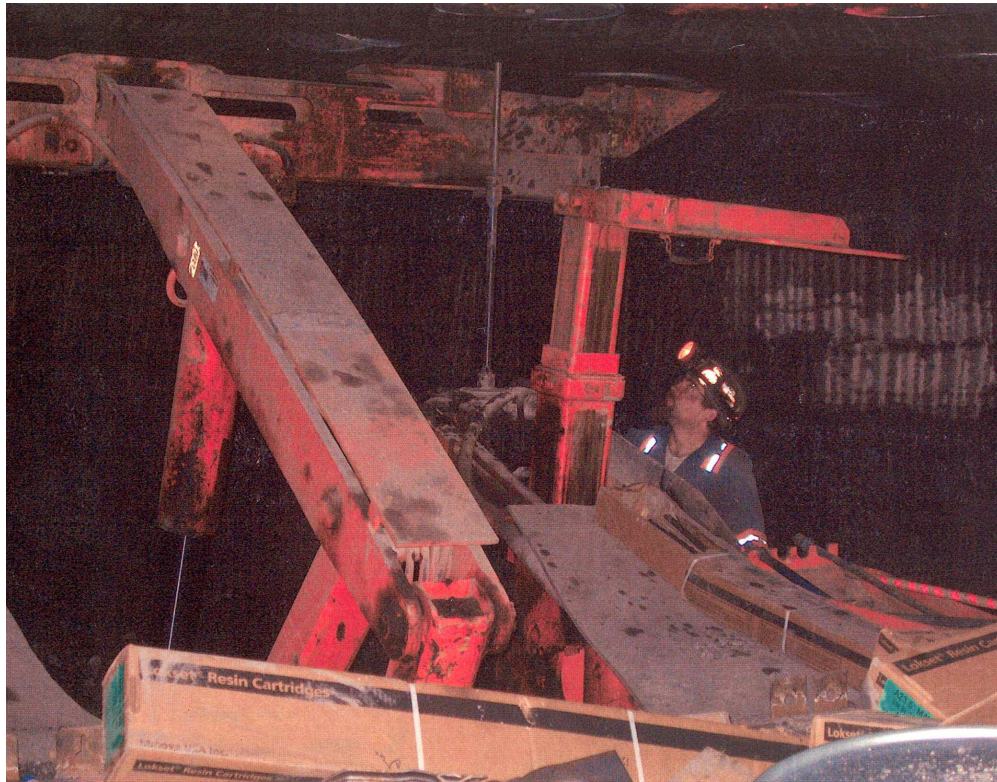
Figure 36 A pinner man runs a roof bolt into the ceiling. Notice the boxes of rosin glue sticks in the foreground and a new pizza pan washer in the bottom right corner. Photo courtesy of Mike.
