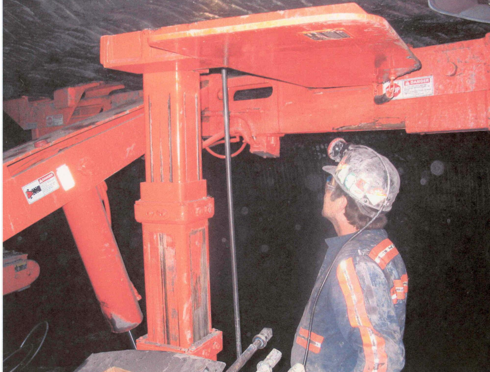
Figure 35 A pinner man drills a hole in the ceiling for a roof bolt. The flat orange “feet” press against the mine roof to support it while the pinner man stands in this newly-mined tunnel. Photo courtesy of Mike.
