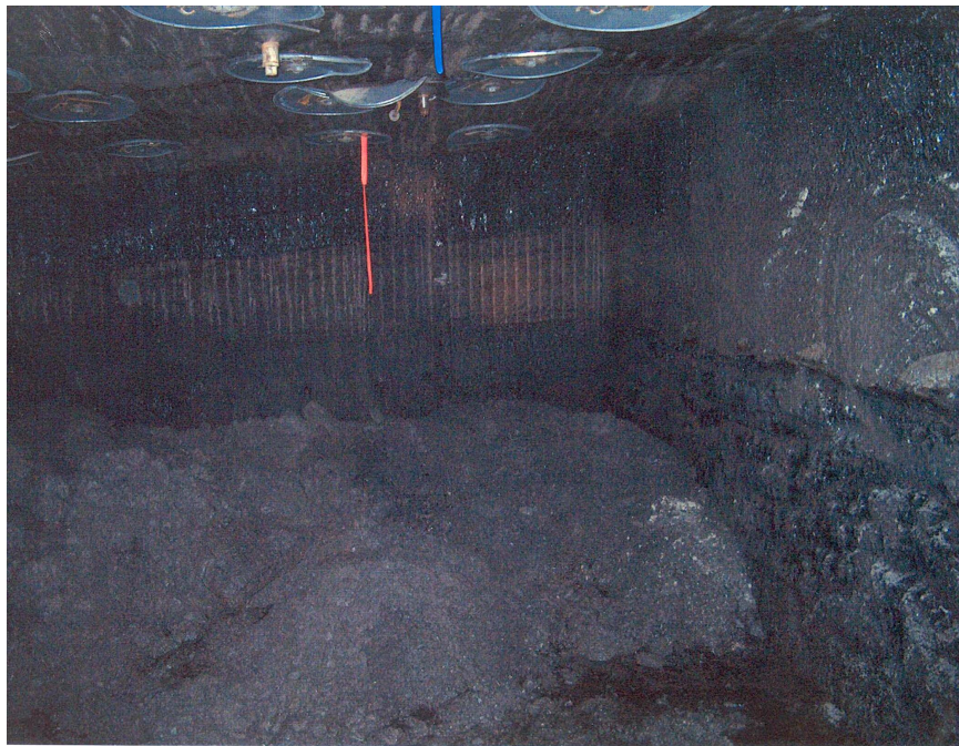
Figure 33 Looking into the face. The miner machine has just been pulled back from this area, and roof bolters have recently installed the roof bolts. The area has not yet been sprayed with white rock dust—notice the score marks from the miner machine's sharp teeth on the face and mine ceiling. Ichabod said that the night shift or hoot owl usually sprays rock dust each night.
