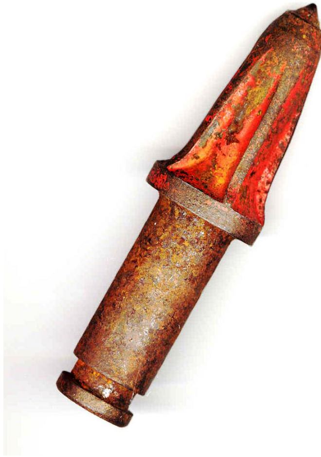
Figure 37 Drill bit from the spinning head of the mining machine. Life-size image. Drill bit courtesy of Bill Buchanan. Photo taken by the author.
