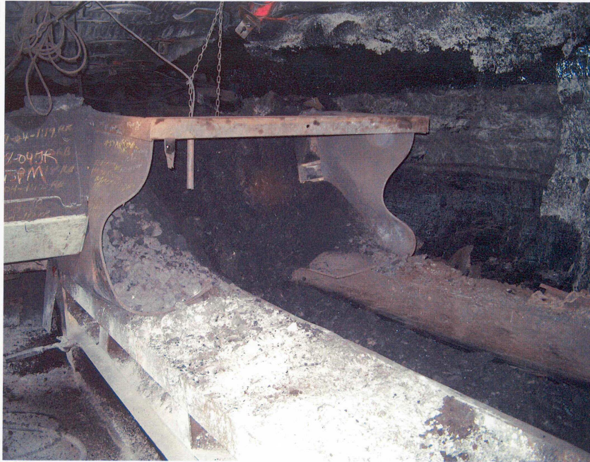
Figure 31 On the other side of the grinding wheel, the chopped coal lands onto the moving belt. This camera angle points towards the face of the mines (away from the mine entrance). Photo courtesy of Mike.
