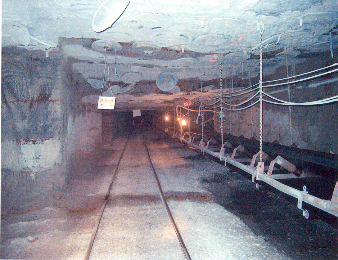
Figure 26 Inside Deep Mine 36. Rails for the man trip run along the center of this photo. The belt is to the right, conveying towards the viewer. The ceiling is coated in white rock dust, and some “pie pans” or “pizza pans” hang down, attached to the roof bolts which support the roof. Photo courtesy of Mike.
