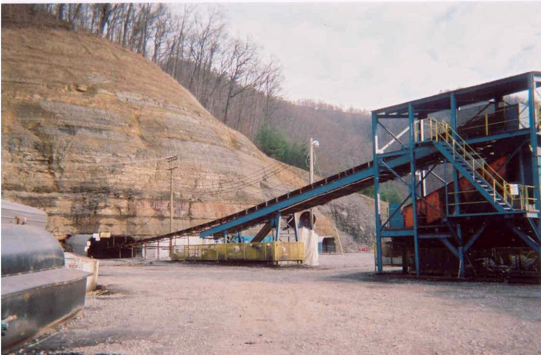
Figure 24 Outside Deep Mine 36. The beltline stretches up to the tippel, which spews coal into trucks (off frame to the right). Photo by the author.
