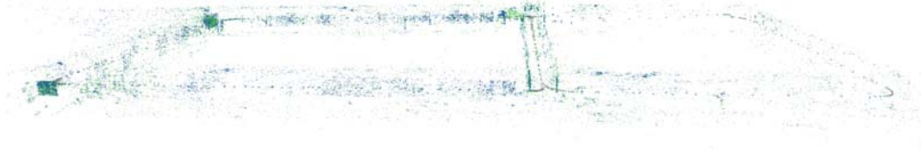
Figure 5.11: The final hallway sequence model viewed from the side. Note that the model is planar matching the planar structure of the building. Green points are differentially tracked scene-flow feature and blue points are SIFT features.
