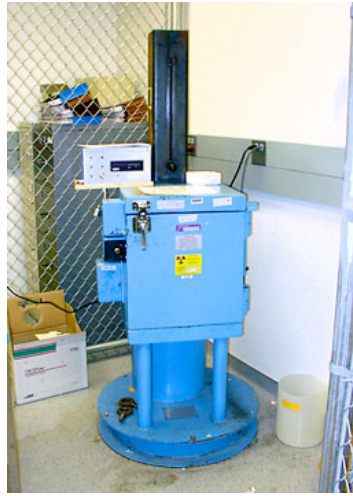
Figure 1.3: J.L. Shepherd Mark 1 Model 30 Cesium Irradiator for irradiation of biological samples. Reproduced from: http://www.immunology.umn.edu/
