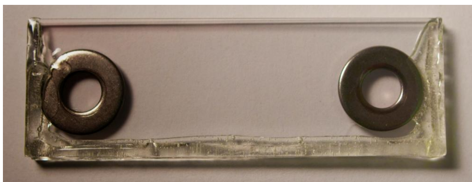
Figure A7.1: Home-made cuvette used to contain dye-sensitized films during transient grating experiments.
