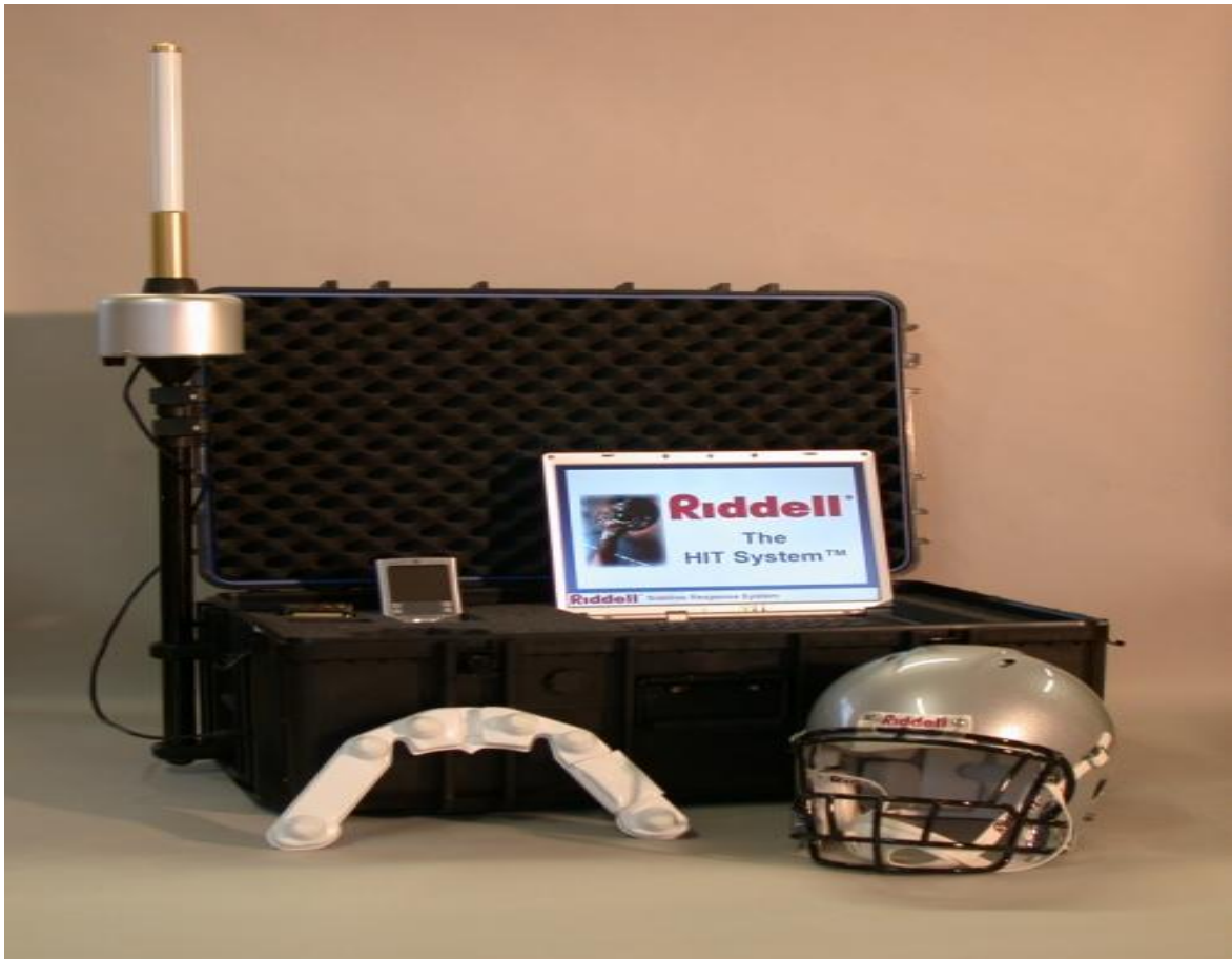
Figure 2: Sideline control unit that stores and displays the information collected. Along side the control is the accelerometer unit and a Riddell helmet which the accelerometer fits into.
