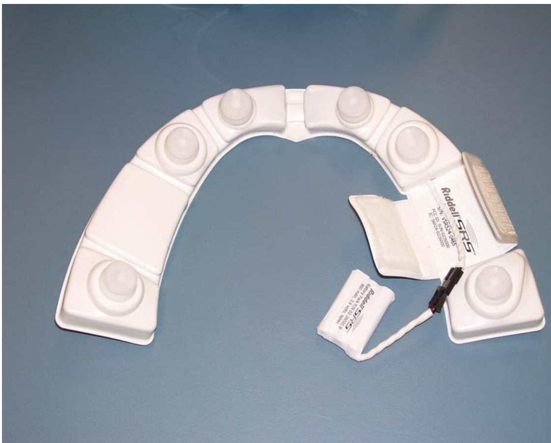
Figure 1: Accelerometer that fits into the Riddell Helmets with battery pack exposed.
