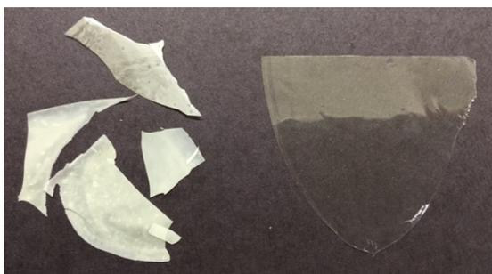
**Figure 4.5** Photograph comparing PETG<sub>2k</sub> (left) to PETG<sub>2k</sub>-H-UPy (right).
