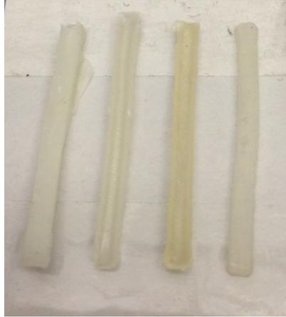
**Figure B21.** Photo depicting minimal discoloration due to UV curing. From left to right: PCL, 35%I, 25%I, 15%I.
