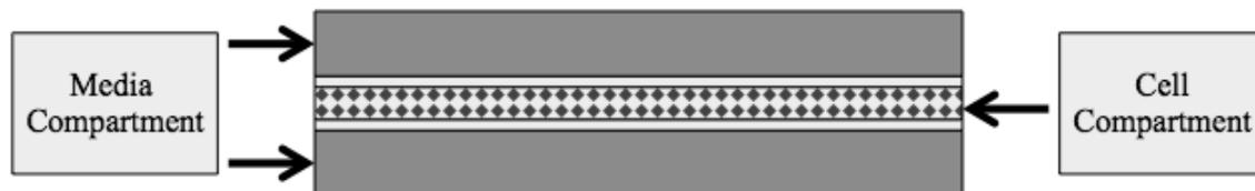
The middle compartment is where the cell culture will be housed, whereas the two outside compartments will where the media flow will pass through. The size and shape of the individual compartments is what is most important. In order to assure that the media will come into contact with the cells, the cross-sectional area of the media compartment is larger than the cell compartment. As far as the shape of the compartments is concerned, it can be described as a teardrop shape.
