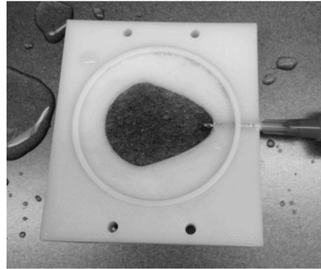
while the other side lies open allows a vacuum-sealed inoculation; as the mixture of media and cells is placed into the cell chamber, the excess media is suctioned out through the PES filter. This method could be done without the use of a vacuum, but it would take considerably longer as the media would have to diffuse out on its own. Nonetheless, with this technique, the chamber was inoculated very evenly and fairly packed.
