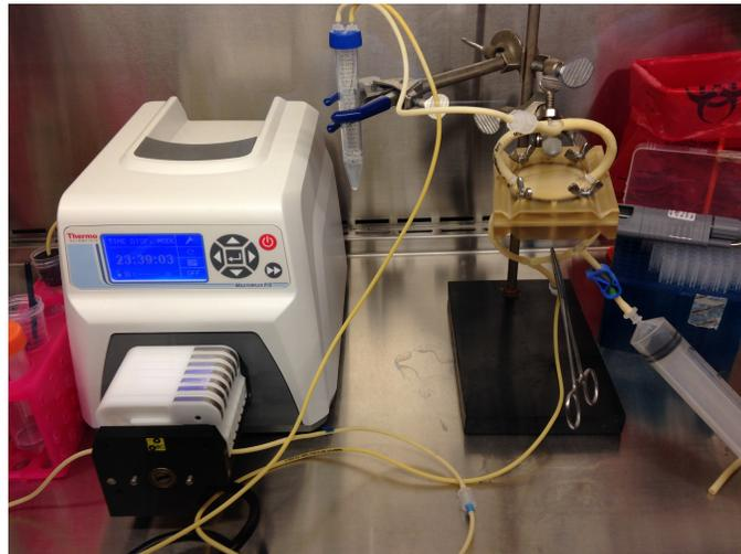
Unfortunately, this initial experiment resulted in the clogging of the filter pores. In the dead ended flow configuration, there was too much albumin produced in the cell chamber, with very little time to diffuse out. However, this is not a major set back, as this just shows that in the dead-ended flow configuration, it is required that the filter pore size be much larger to accommodate for the induced radial flow. Initial results from the first
