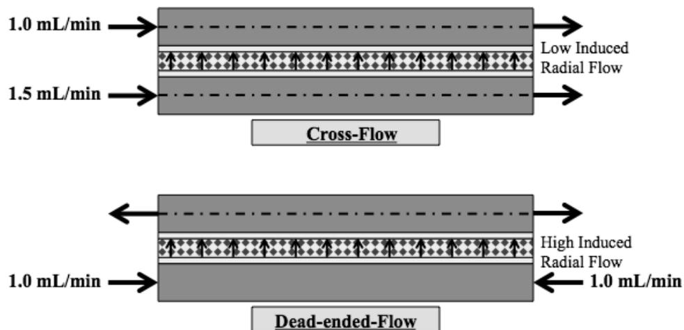
The ability to run experiments in different flow configurations is not vital, however, it allows for more flexibility in the types of experiments that can be run. The ability to pressurize one side of the bioreactor at a time also allows for better inoculation technique. By attaching a lab vacuum to both inlet and outlet of one media compartment
