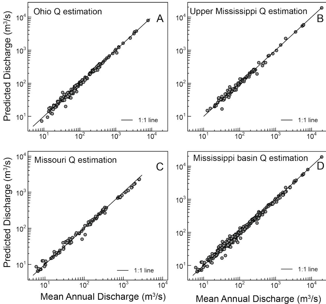
**Figure 10:** Estimated and USGS measured mean discharges for 346 gauging stations in the Mississippi basin.
