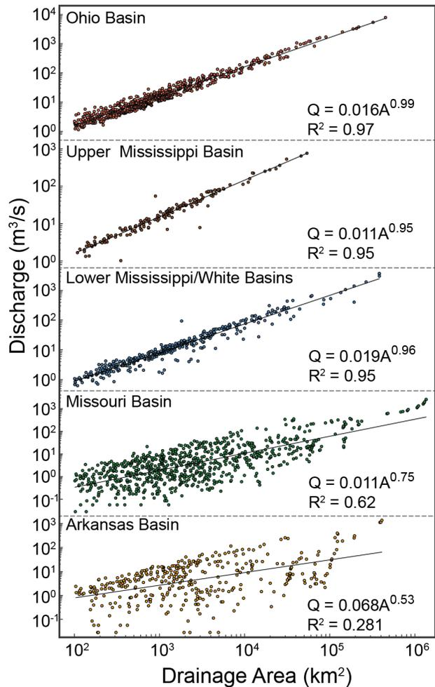
**Figure 3:** Discharge-drainage area relationships for sub-basins of the Mississippi; exponents close to one indicate a nearly linear fit in the Ohio, Upper and Lower Mississippi sub-basins, but there is substantial deviation from unity in the Missouri and Arkansas sub-basins.
