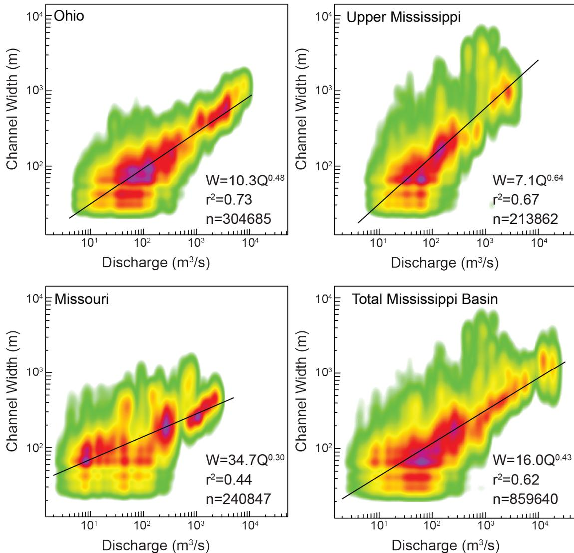
**Figure 11:** Density plots of width versus discharge for the Ohio, Upper Mississippi, Missouri, and entire Mississippi basin. Linear fits represent downstream hydraulic geometry relationships analogous to Equation 1a.
