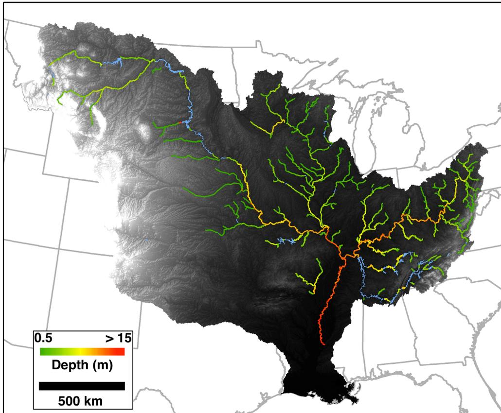
**Figure 12:**  $8 \times 10^5$  mean depths in the Mississippi basin estimated using multiple regression of  $d$  against  $Q$  and  $w$ ; lakes shown in blue.
