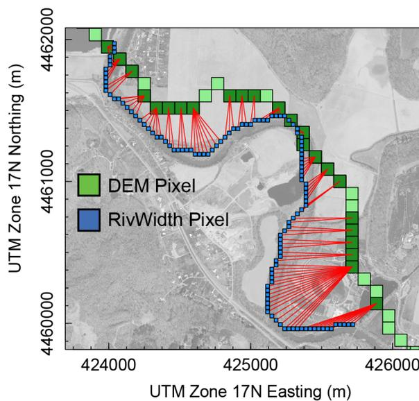
**Figure 4:** Linking RivWidth and DEM measurements; RivWidth measurements for the Walhonding River near Coshcocton, PA, matched to the nearest downstream DEM-derived channel pixels with drainage area values.
