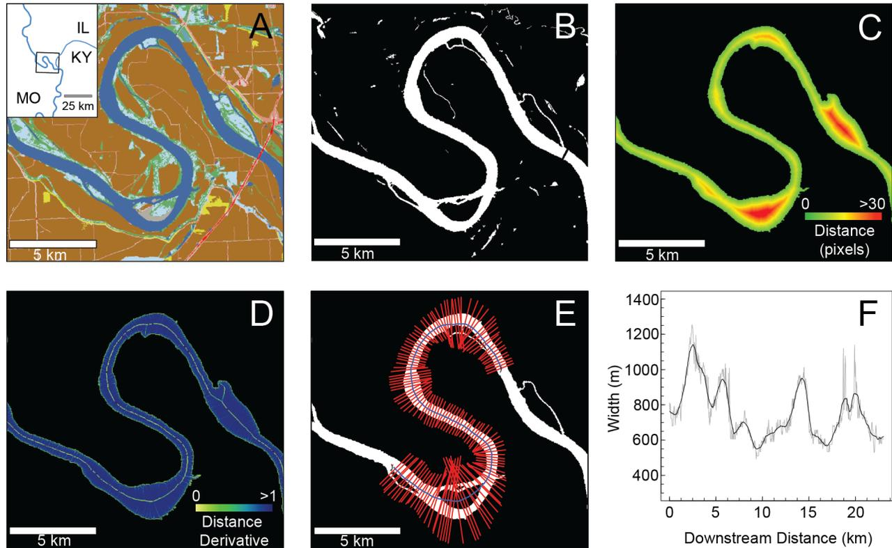
**Figure 2:** Inputs, intermediate steps, and products for calculation of river width in this study: A) National Land Cover Dataset; B) binary water mask of the open water classification; C) distance image based on a filled channel mask; D) derivative of distance image used to calculate the centerline; E) flow width measurements along orthogonal line segments to each centerline pixel; F) plot of raw (grey) and smoothed (black) continuous widths.
