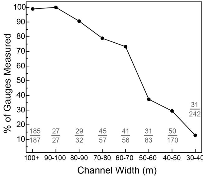
**Figure 7:** Percentage of USGS gauging stations measured in this study, binned by *in situ* channel width; grey fractions indicate number measured out of total gauges per 10-m width range.
