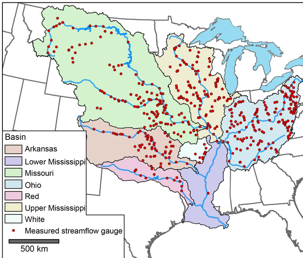
**Figure 1:** Major sub-basins of the Mississippi and USGS gauging stations used for width validation.
