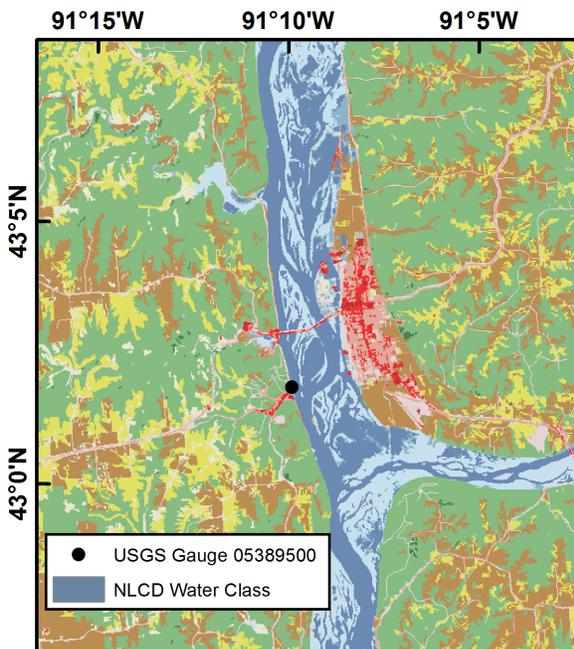
**Figure 9:** NLCD image of the Upper Mississippi River near MacGregor, IA; inundated floodplains are extensively connected to channels, leading to high width error.
