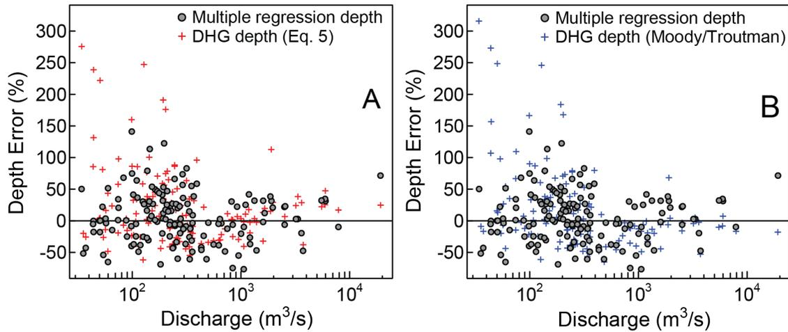
**Figure 13:** Relative depth error for multiple regression method (circles) and A) DHG estimate (this study); B) DHG estimate (Moody and Troutman, 2002).
