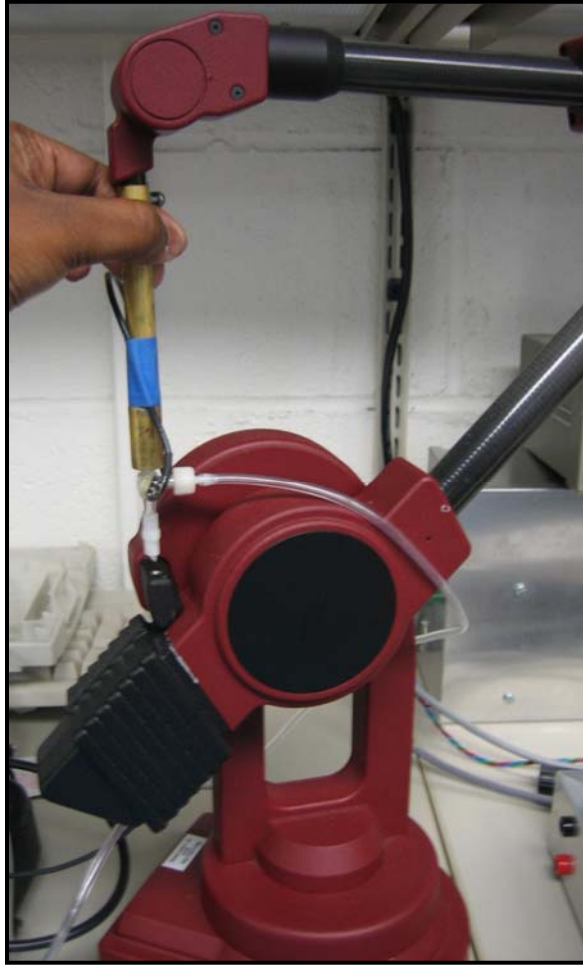
Figure 4.11: Electrode probe and digitizer
