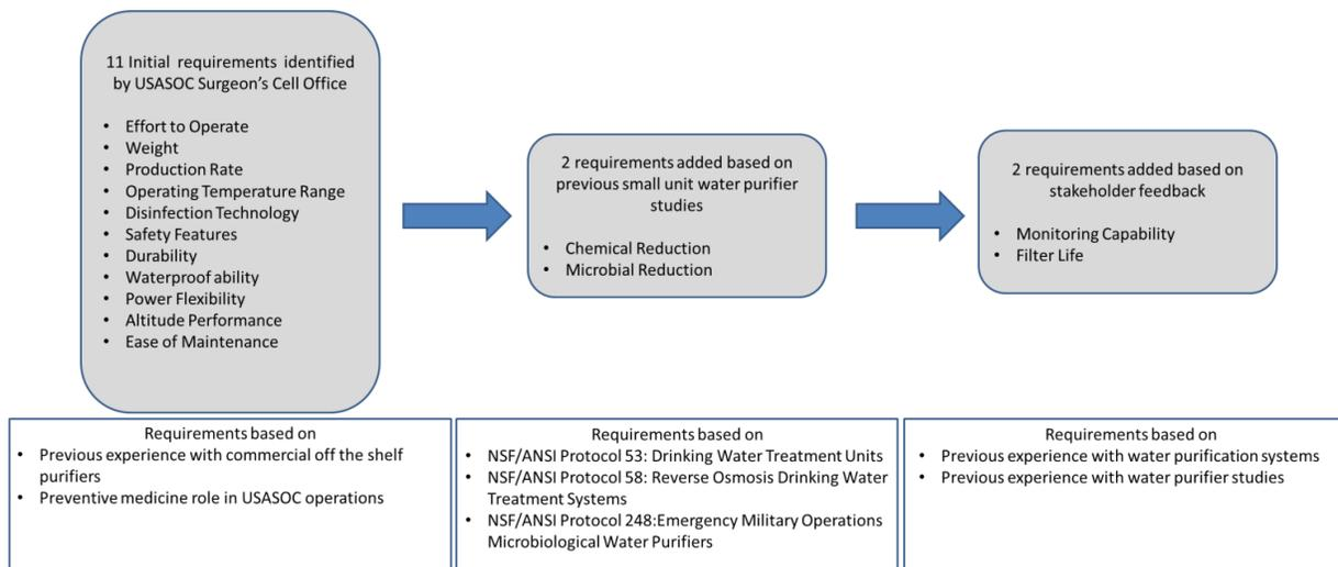
**Figure 4.** Requirement identification process
