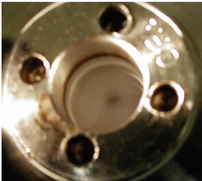
Figure 4.3: Milk-like suspension in the pseudo-dispersion polymerization of MMA in \text{scCO}_2 .
