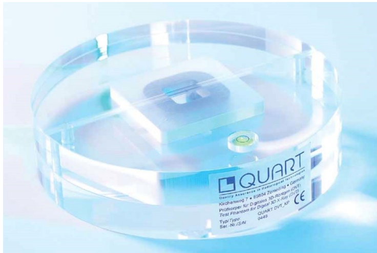
Figure 3. QUART DVT_AP phantom.
