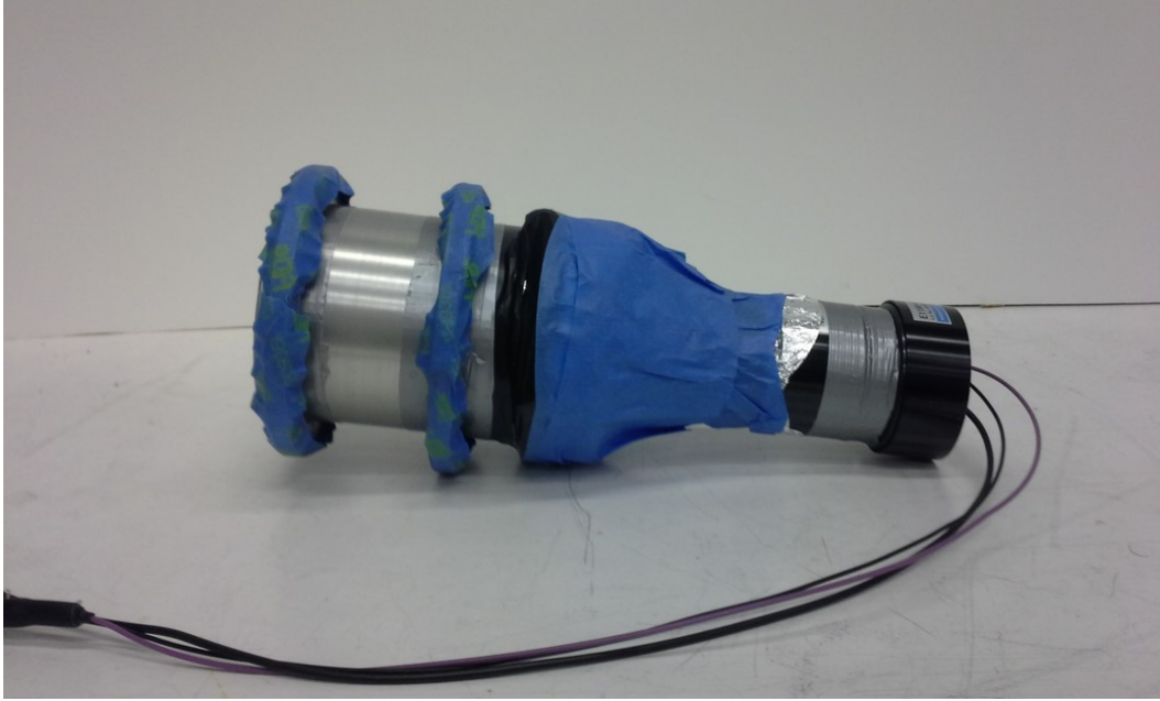
Figure 5.5: BC-523A boron-doped liquid scintillator. Blue tape was used to electrically insulate segments, and aluminum foil was used to electrically ground segments.
