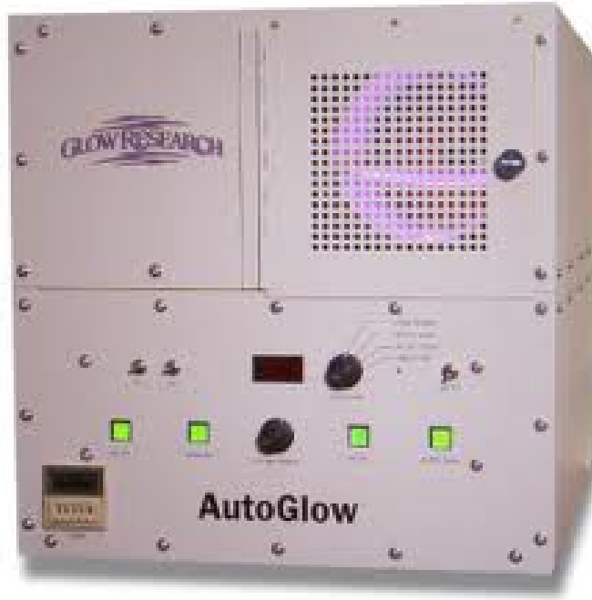
Figure 4.7: The Grow Research AutoGlow plasma cleaner used to eliminate carbon.
