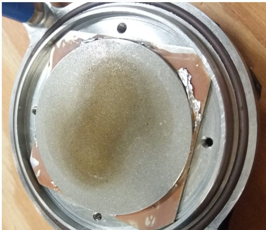
Figure 4.17: Sintered titanium target. The round disk is the sintered titanium backing, and the irregular dark spot on the surface is the region with implanted ^{22}\text{Ne} atoms. The brown square around the disc is epoxy affixing it to the square nickel sheet. The target holder is seen behind the target.
