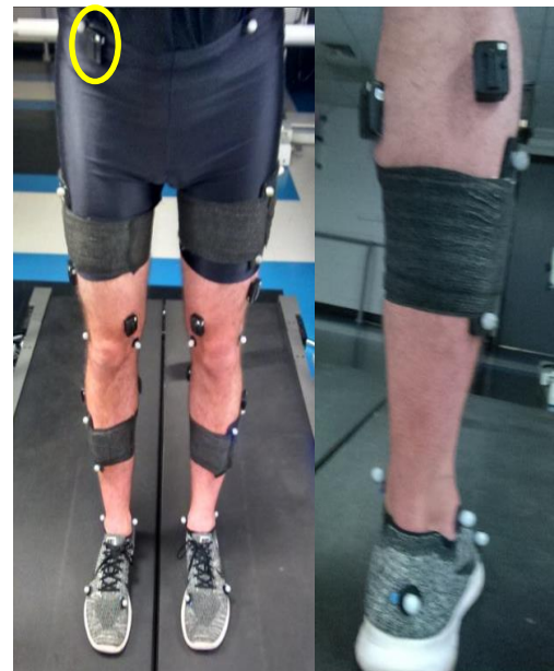
Figure 5.7: Experimental kinematic marker and electromyography sensors marker set-up for running and hopping protocol. Waist mounted accelerometer noted in yellow circle.
