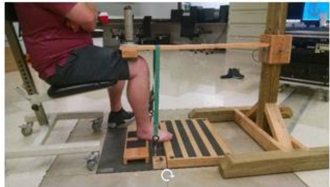
Figure 5.2: Experimental set-up for ankle plantarflexion MVIC with ankle joint in neutral position
