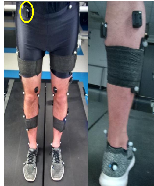
Figure 3.7: Experimental kinematic marker and electromyography sensors marker set-up for running and hopping protocol. Waist mounted accelerometer noted in yellow circle.
