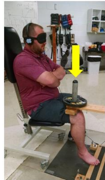
Figure 3.2: Experimental set-up for ankle plantarflexion MTS. Downward perturbation noted by arrow.
