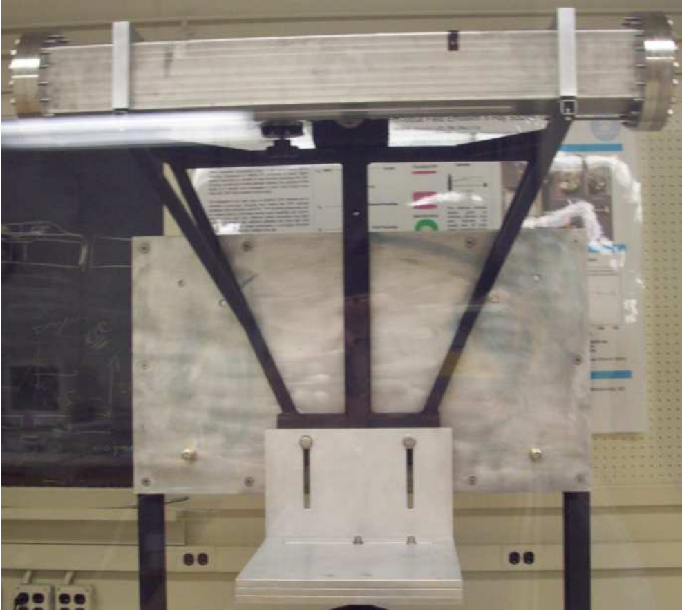
Figure 10: Mounting structure with chamber
