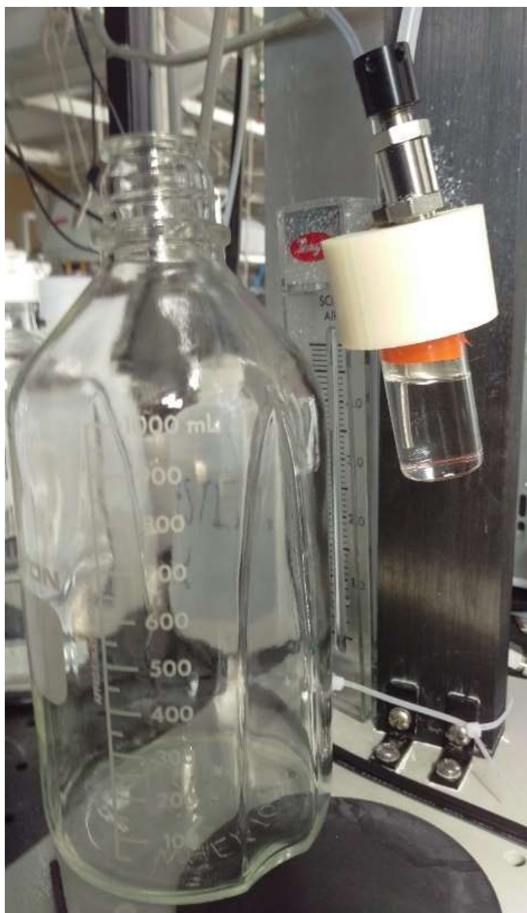
Figure 2.3. COA with 3D printed cap on 20 mL scintillation vial in operation.
