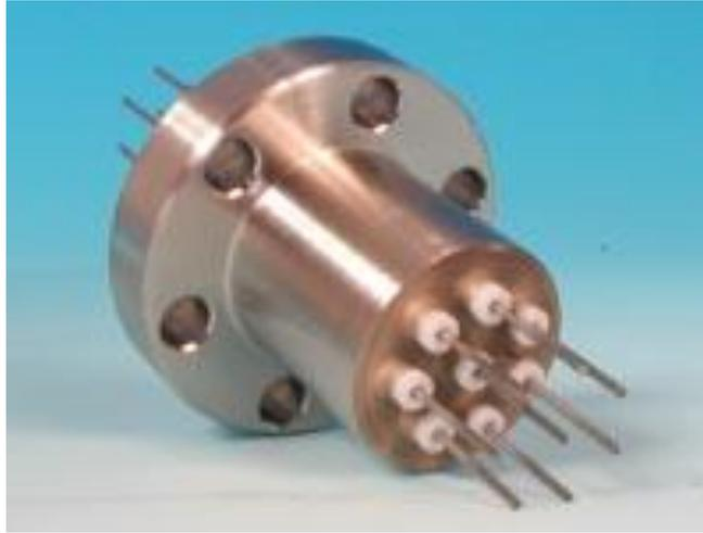
Figure 3.4.2 Picture of the commercial feedthrough purchased from MDC Vacuum Products Corporation. It is attached to the end of the TEM holder shaft, connecting the 8 electrical wires inside the holder to the power supply outside the TEM.
