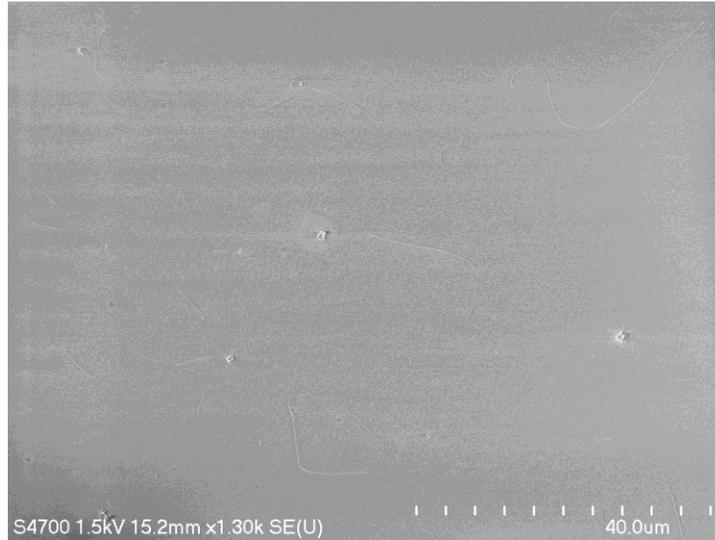
Figure 3.3.1 SEM image of SWNTs using Fe/Mo nano-particles as catalysts.
