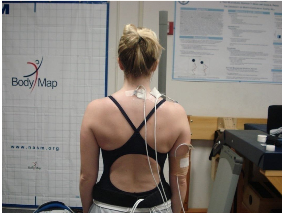
Figure 1. Electromagnetic tracking sensor placement
