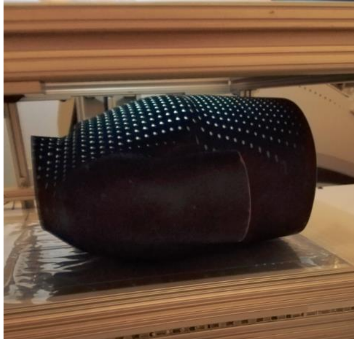
Figure 5-29: Photo of the anthropomorphic thoracic phantom situated for PSD imaging.
