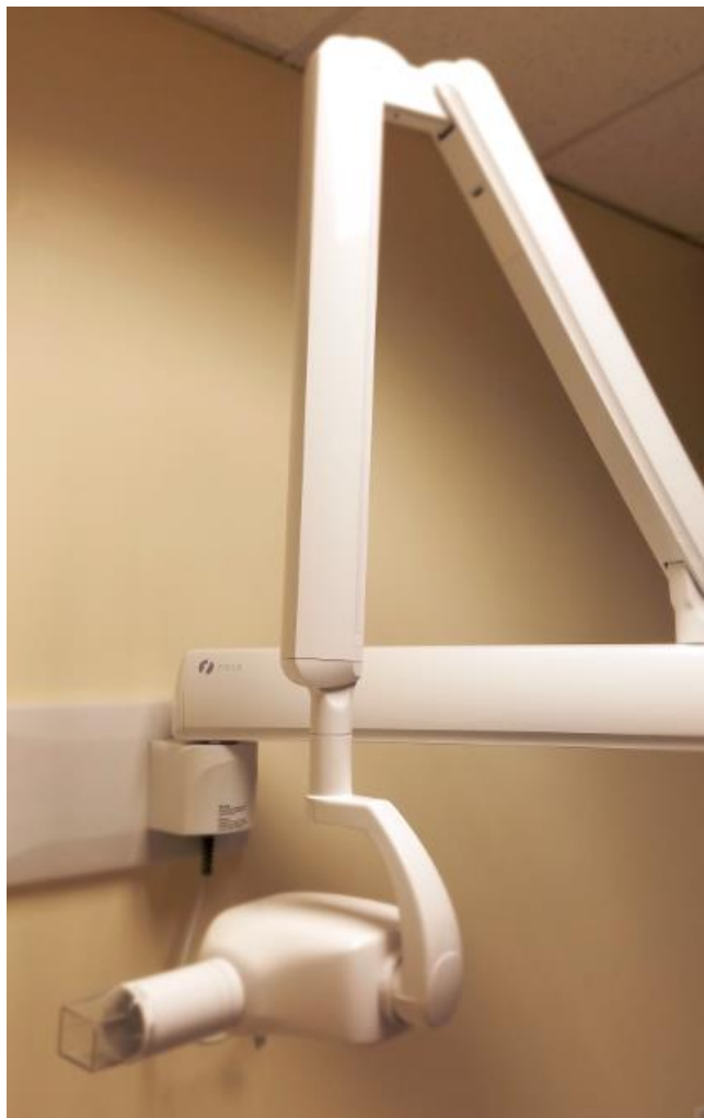
Figure 3-14: 2D intraoral system (a) used for dose validation with ion chamber positioning for entrance (b) and exit (c) dose measurement.
