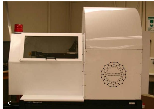
Figure 2-1: a) An early CNT x-ray source constructed in a large vacuum chamber; b) A CNT-based micro-focus x-ray tube incorporated into (c) a micro-CT system with integrated shielding for small animal imaging designed and constructed at UNC.
