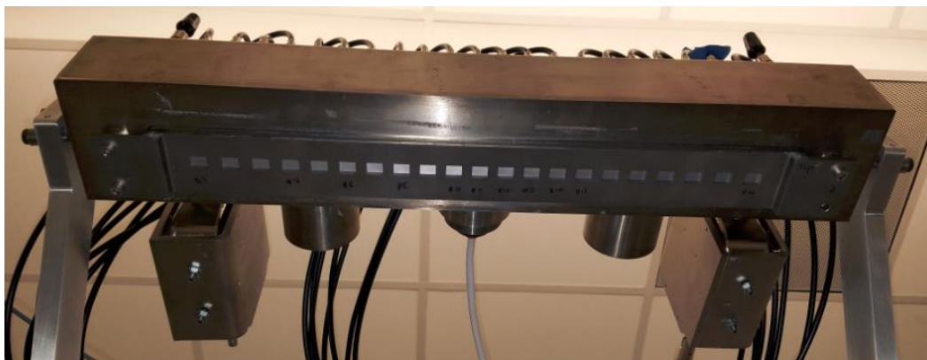
Figure 2-3: a) Photo of two of the first CNT linear x-ray source arrays fabricated in our lab at UNC; b) Photo of a recently fabricated CNT x-ray source array from Xinray Systems.
