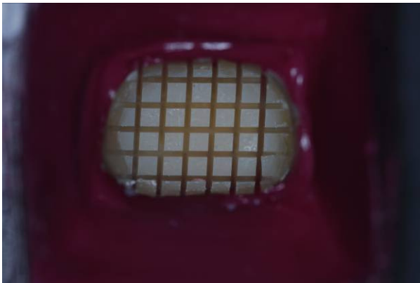
Figure 11. Specimens sectioned into rods of approximately 1x1 mm.
