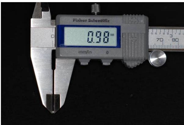
Figure 13. Measurement of dentin-composite interface with a digital caliper.
