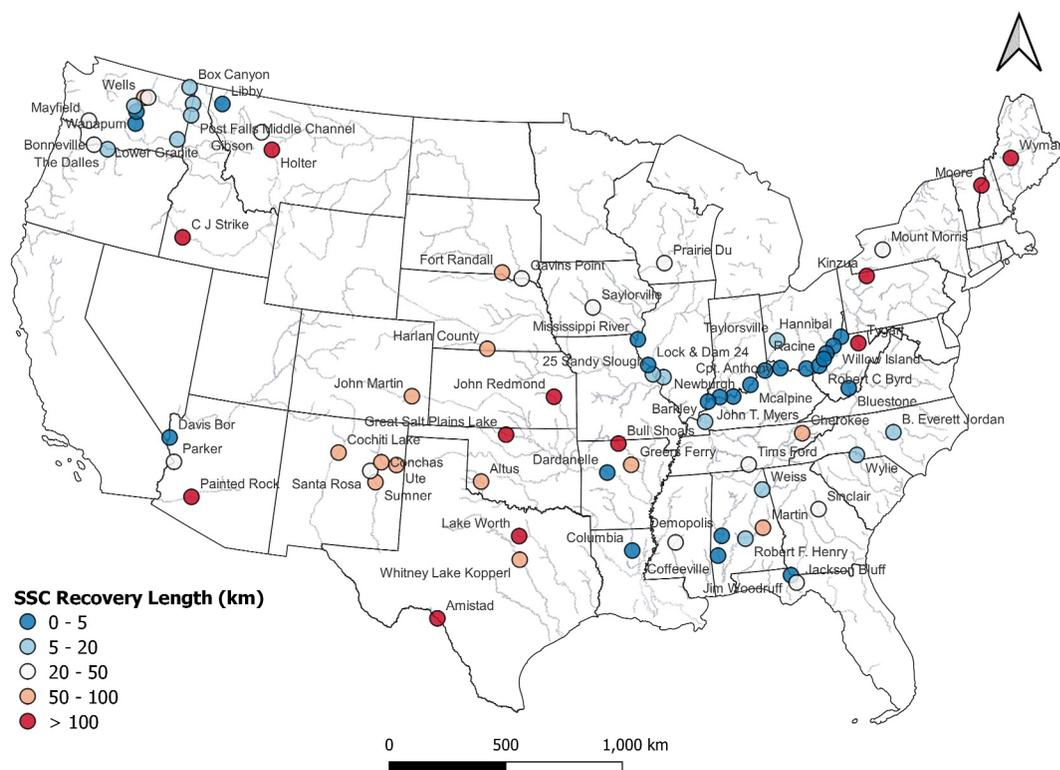
**Figure 2.** Map of dam locations and suspended sediment concentration recovery lengths for dams with 100% recovery. Blue circles are dams with the shortest recovery lengths, while dams with the highest recovery lengths are shown in red circles.
