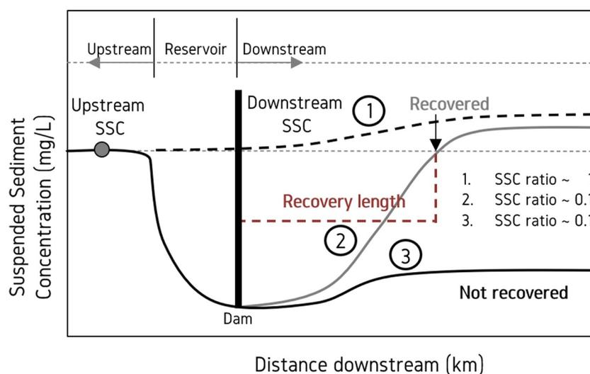
**Figure 1.** Schematic diagram for suspended sediment concentration (SSC) recovery. The SSC ratio is the ratio of SSC of the river segment just downstream of the dam to reference SSC upstream of the reservoir. SSC ratio is  $\sim 1$  for case 1, as SSC downstream of dam and SSC upstream of the reservoir are similar whereas SSC ratio for cases 2 and 3 are less than 1 as downstream SSC is smaller than upstream SSC.
