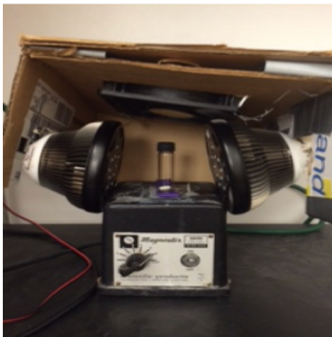
Figure 3.19: Photoreactor setup used for halofunctionalization reactions. Reaction vials were placed about 5 cm from the face of both lamps. Above a simple fan was used to cool the reaction.
