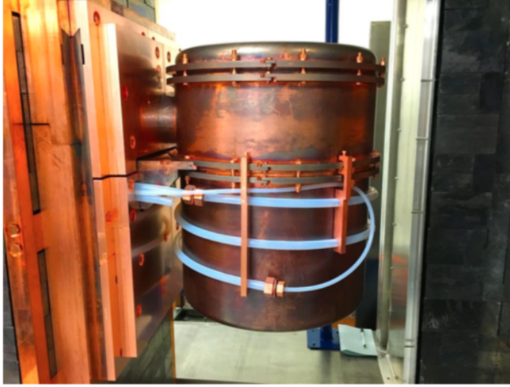
Figure 3.13: The DEMONSTRATOR calibration system. A line source is inserted via the clear plastic tubing track through the shield, at left. The track source wraps helically around the copper cryostat.
