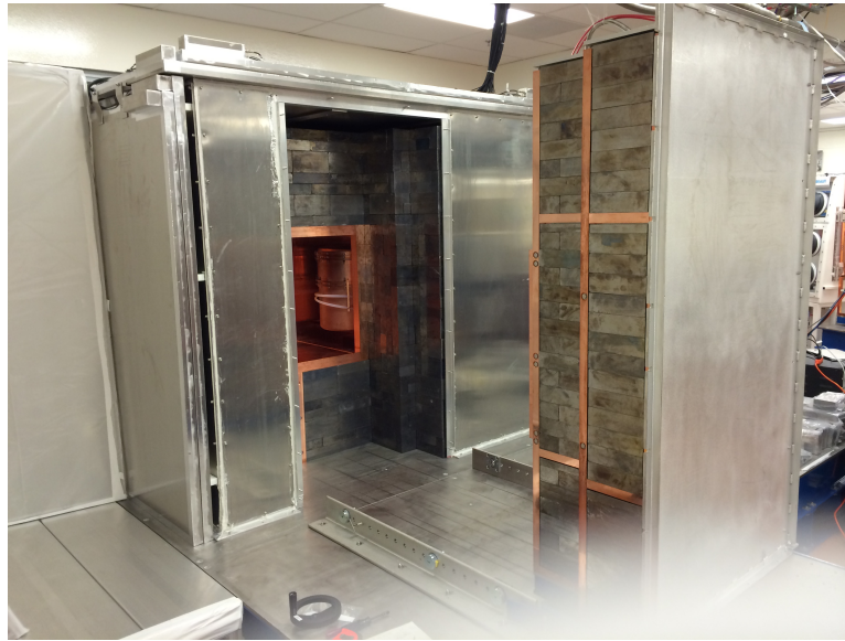
Figure 1.3: (a) A schematic of the DEMONSTRATOR shield. (b) A picture of the shield components up to the Radon enclosure. A cryostat is visible inside the shield. The removable “blank” monolith seen here pulled away from the shield has been replaced with a second cryostat, and both modules are currently taking data.
