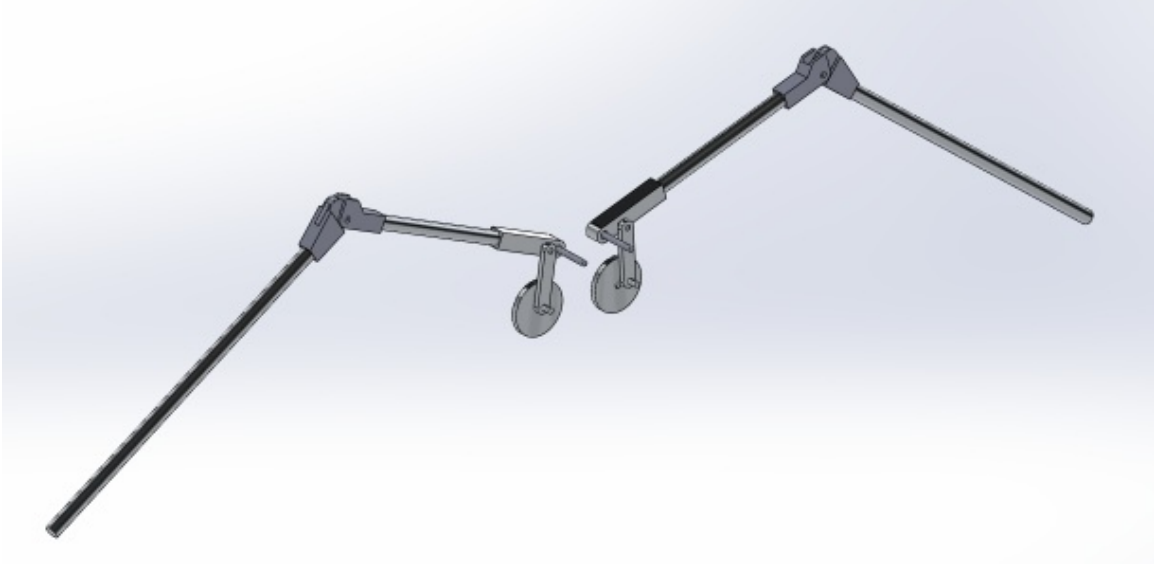
Figure 2.1: Assembly for simulating flapping of a passive joint in SolidWorks
