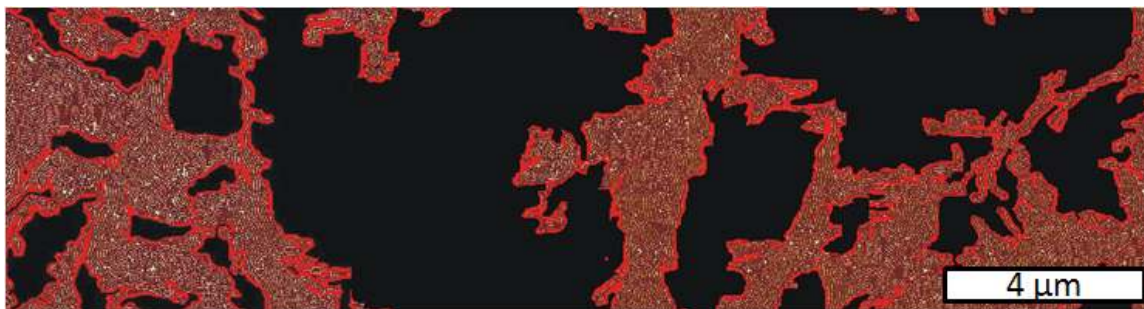
Figure 3.13 Images of networks. AFM images of a large span of surface. The networks are lined with red and blacked out to make them easy to see. The sizes of the individual networks can grow greater than 25\ \mu\text{m}^2 .
