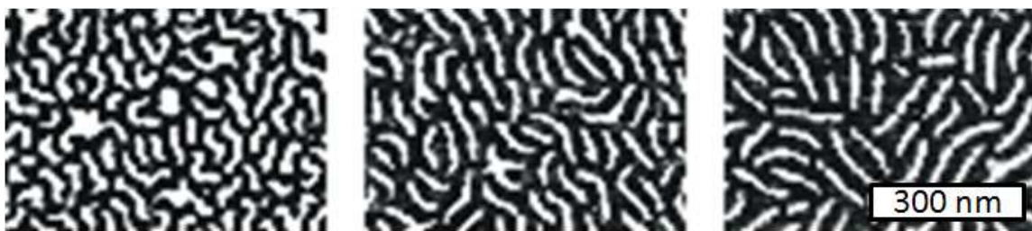
Figure 2.4 Images of brush molecules at various film pressures. The molecules all have the same dimensions, N = 500 and n = 35 . The highest surface pressure \sim 18 mN/m is on the left side while the lowest \sim 1 mN/m is on the right side.
