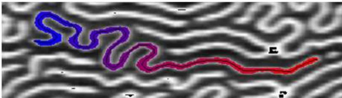
Figure 2.8 Diagram of molecular analysis. A polymer brush molecule isolated by the Pen program. The contour is traced.
