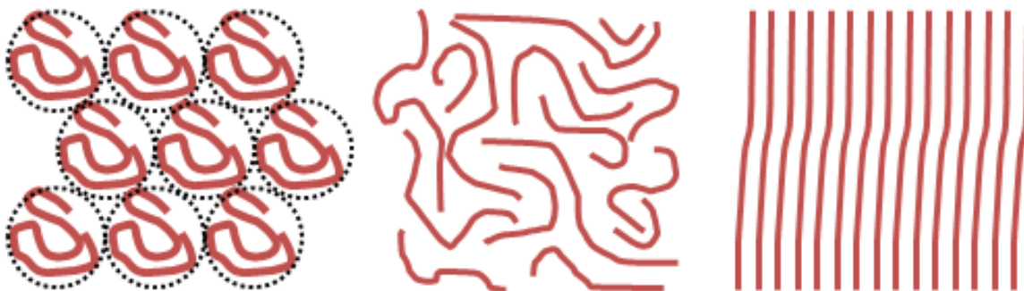
Figure 3.11 Packing arrangements. The various packing arrangement that are possible in the monolayer systems: a collapsed disk-like packing (left), an ideal packing in a self-avoiding 2D walk (center), and an extended packing (right).
