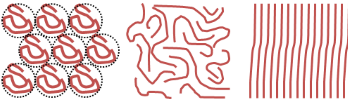
Figure 1.2 Different packing arrangements and conformations of polymer molecules. Collapsed and separated (left), coiled and blended (center), and extended and aligned (right).
