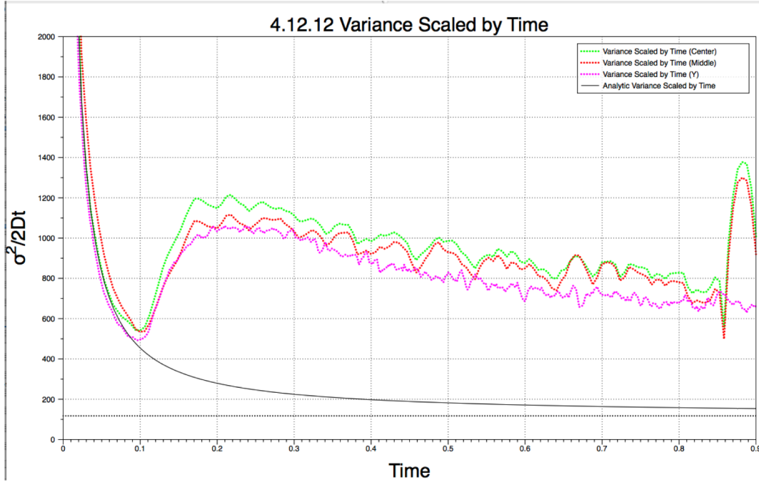
Figure 7.10: The chart above shows the Normalized Variance (Non-Dimensional) vs. Time (Non-Dimensional). The Normalized Variance plots are shown for the Center and Middle Partial Planar Slices, the Y-Average, and the Analytic Solution. This data represents all 450 images (7 minutes, 30 seconds elapsed time) of the data set taken on 4/12/12.
