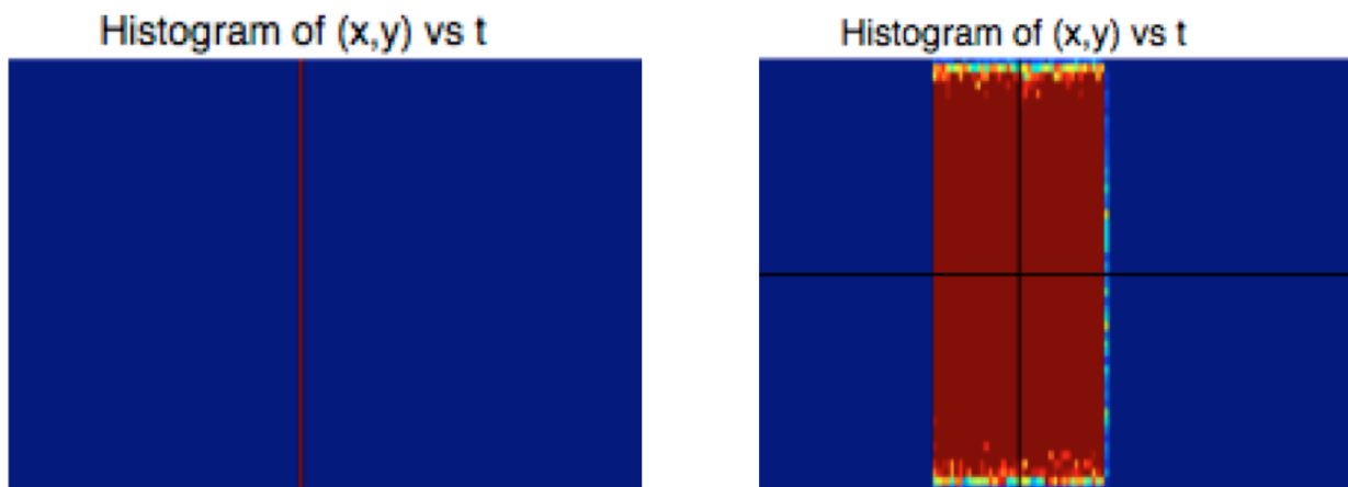
Figure 5.2: This figure shows the (x,y) Histogram representation of the initial conditions. The picture on the left represents initial condition 3 which is the vertical disk of dye solute. The picture on the right represents a plug of finite length for the initial condition of the dye solute.
