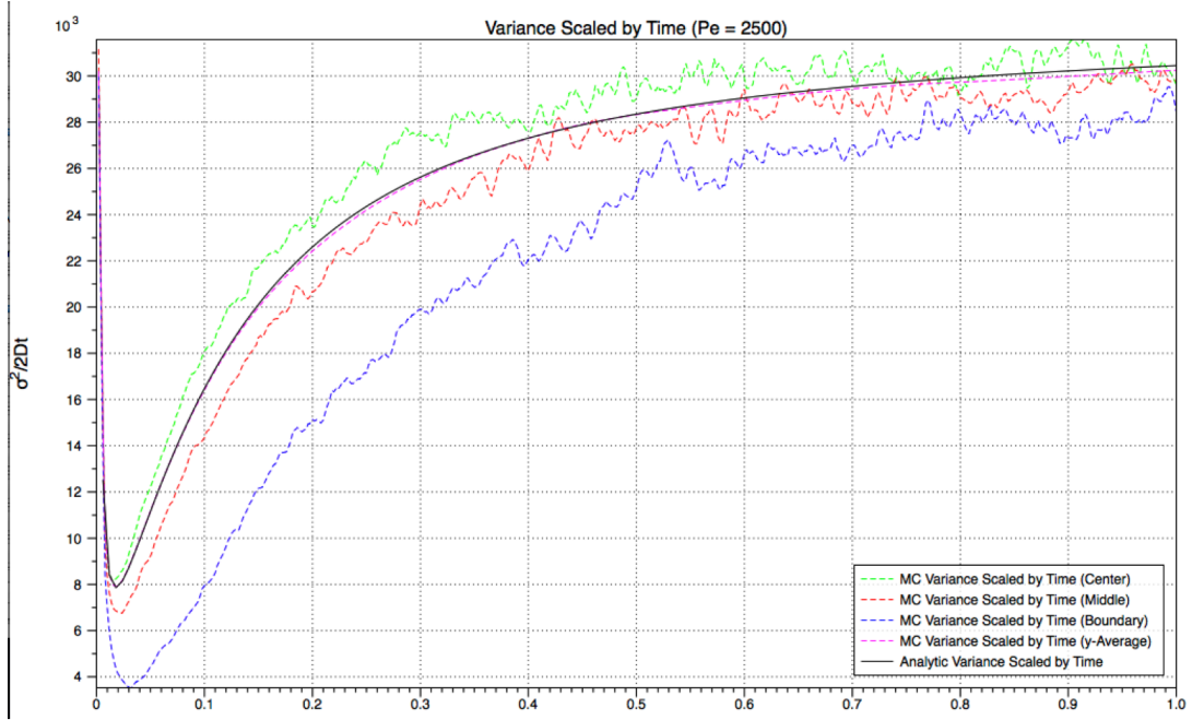
Figure 6.11: This figure shows variance scaled by time on the y-axis and time on the x-axis. This data represents a 2500 Peclet number.
