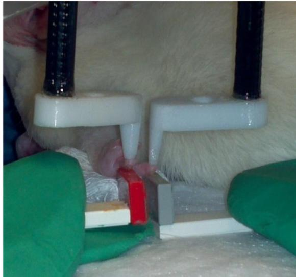
**Figure 1.2: Digit Platform and Stimulus Probe Setup**
