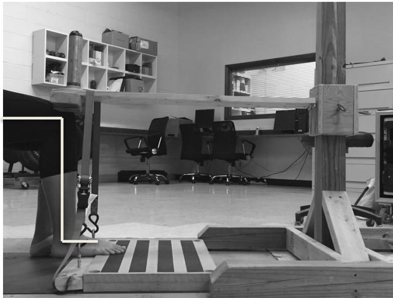
**Figure 3.2 Experimental setup for collecting MVIC data. The participant's hip, knee, and ankle will be flexed to 90 degrees. A strap will hold the perturbation lever in place while the participant maximally contracts their plantarflexor muscles forcing their knee into the lever.**
