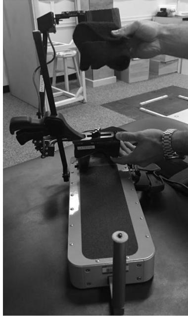
**Figure 3.5: Hollis Ankle Arthrometer**
