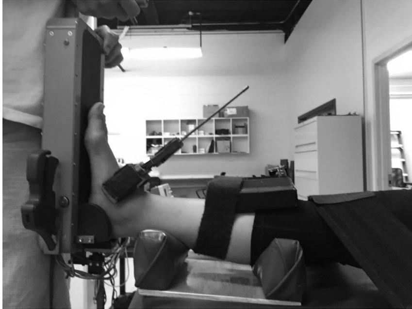
**Figure 3.6: Medial view of Hollis ankle arthrometer set up with straps securing knee and ankle**
