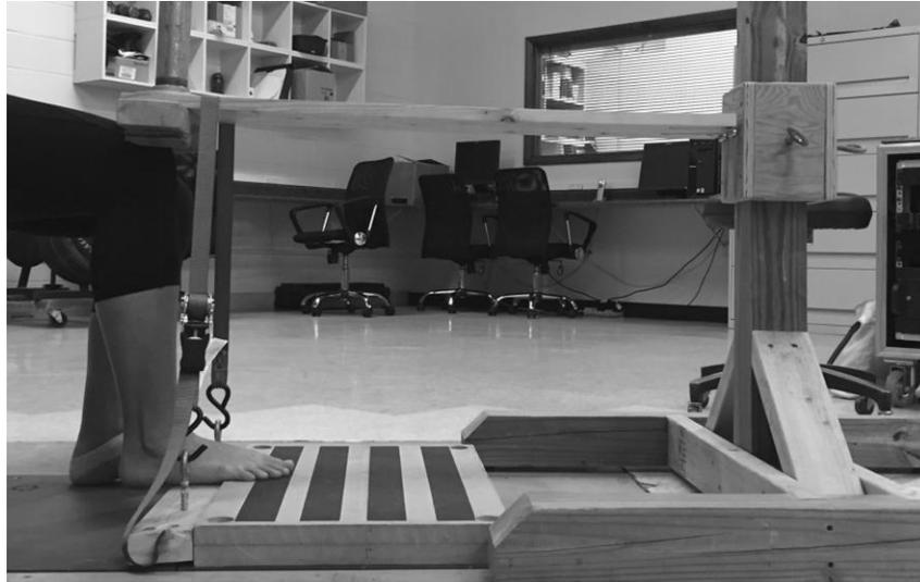
**Figure 4.2 Experimental setup for collecting MVIC data. The participant's hip, knee, and ankle will be flexed to 90 degrees. A strap will hold the perturbation lever in place while the participant maximally contracts their plantarflexor muscles forcing their knee into the lever**
