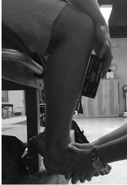
**Figure 4.4: Talar glide measurement with foot in neutral eversion/inversion and plantarflexion/dorsiflexion. A digital inclinometer placed along the tibia inferior to the tibial tuberosity to measure the angle at the restriction point.**
