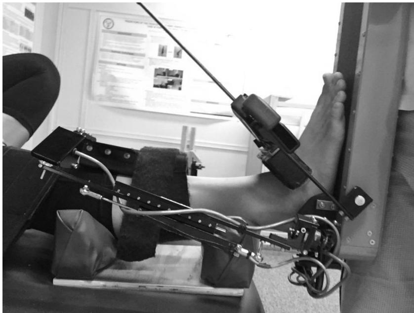
**Figure 3.7: Lateral view of Hollis ankle arthrometer set up.**
