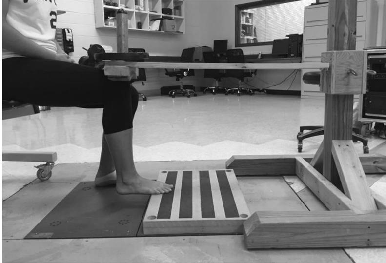
**Figure 4.3: Triceps surae muscle stiffness perturbation device and set up with hip, knee, and ankle at 90 degrees and perturbation lever parallel with ground.**
