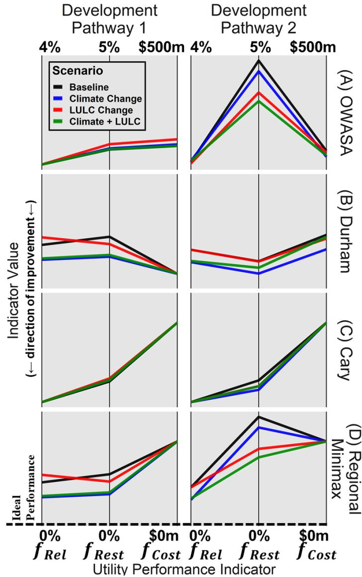
Figure 2.7: Panels of parallel axis plots showing modeled outcomes based on three regional utility performance indicators. Model evaluations under tested hydrologic scenarios (colors) are given for each regional utility and the overall region (rows) for two contrasting development pathways (columns). Each line represents one model evaluation’s performance across each indicator.
