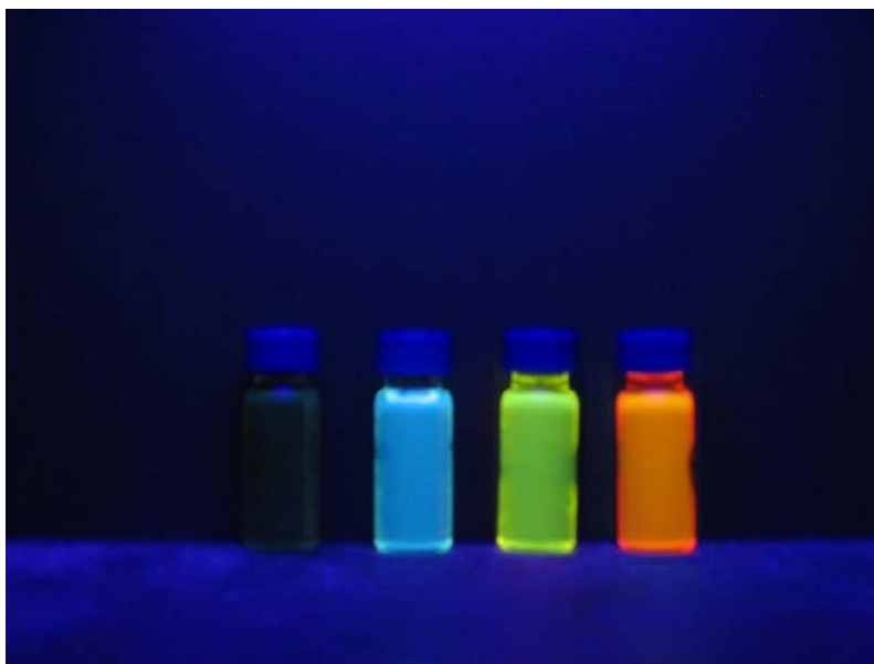
Figure 5.10. Fluorescence of (left to right) P1 , PII , PIII , PIV when exposed to 365 nm light in THF solutions
