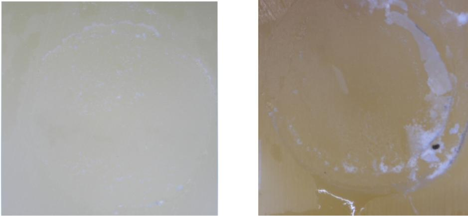
**Figure 11:** Examples of modes of failure in the SBS test **A)** Adhesive **B)** Mixed failure.
