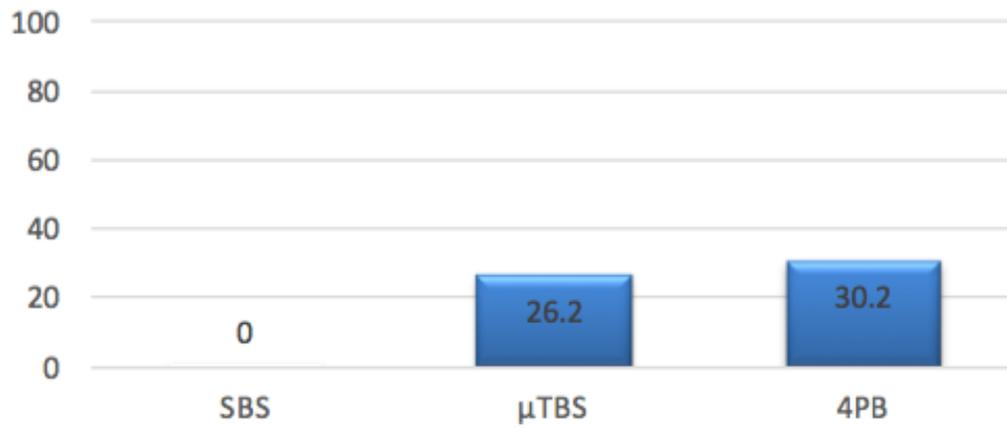
**Figure 8:** Percentage of pre-test failure by test method.
