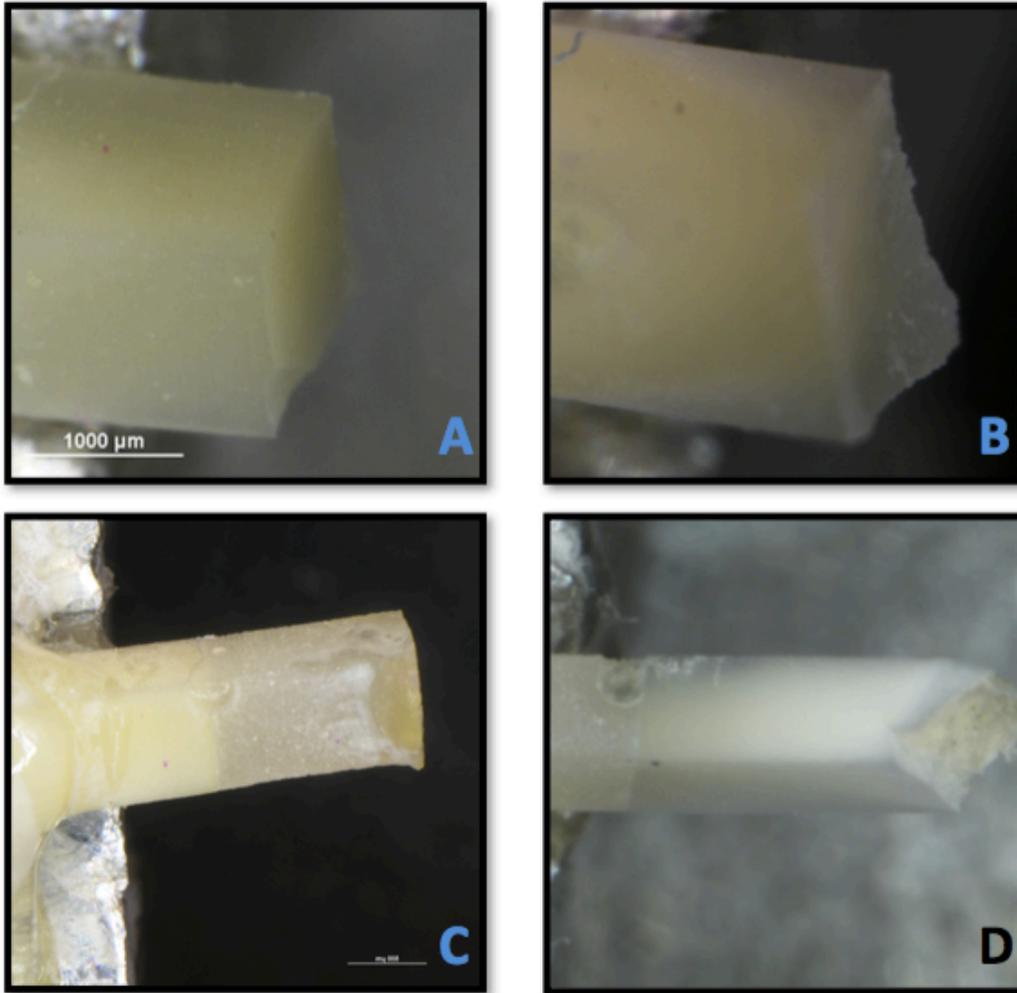
**Figure 12:** Examples of modes of failure in the  $\mu$ TBS and the 4PBBS tests: A) Adhesive, B) Mixed, C) Cohesive in the RMGI D) Cohesive failure in dentin
