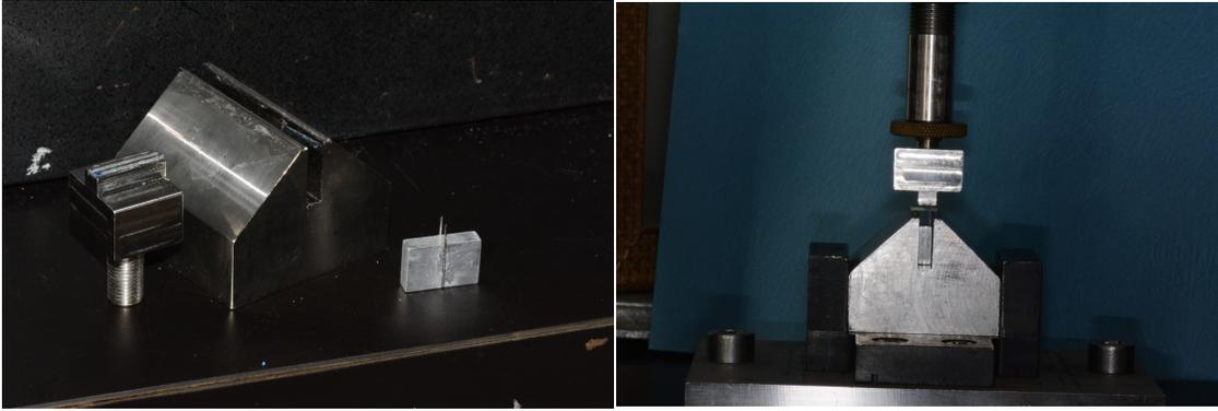
**Figure 7: A) 4-Point Bending test assembly B) A beam mounted in the Instron machine.**
