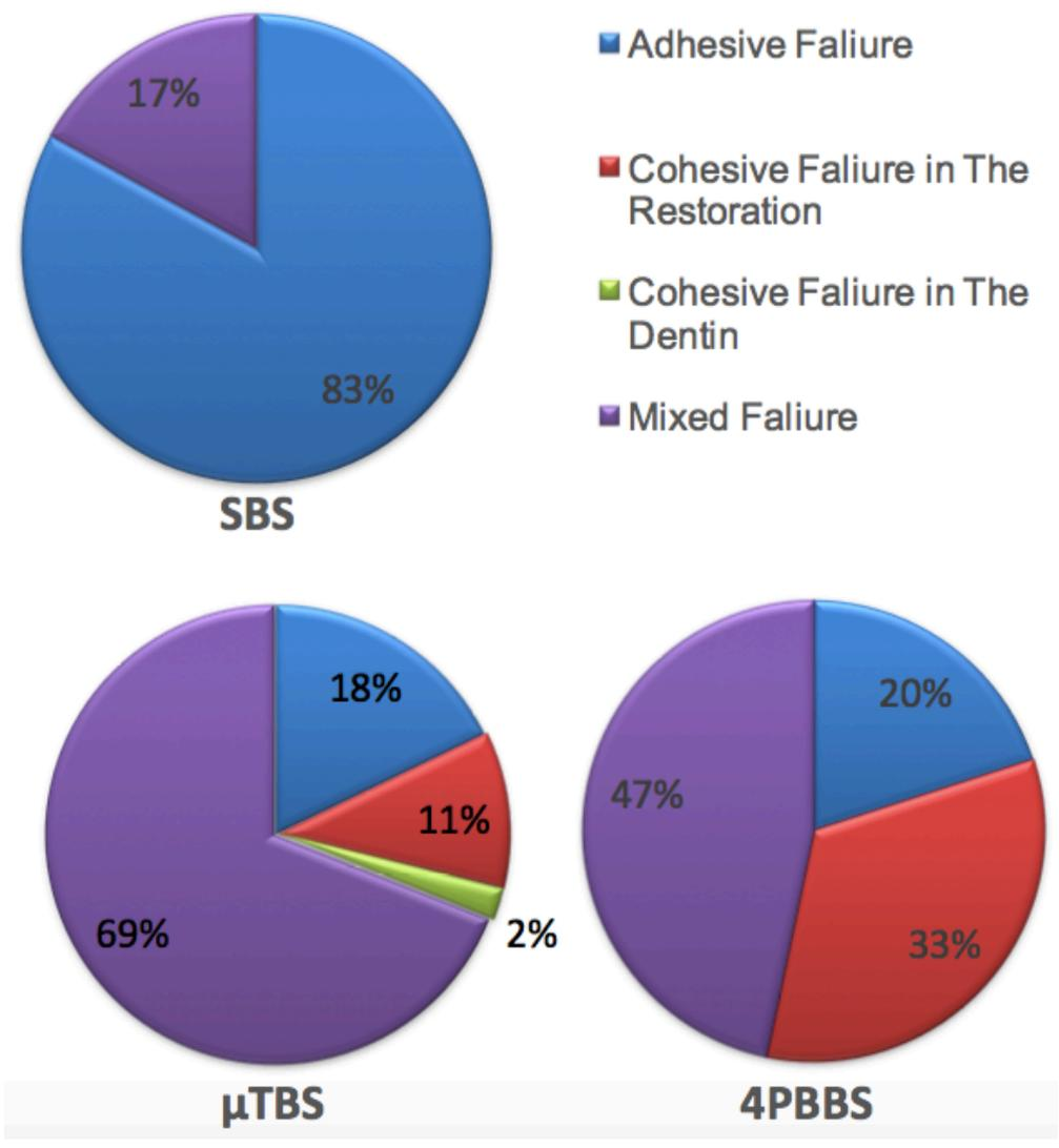
**Figure 10:** Representation of types and relative percentages of modes of Fuji II LC bond failure as observed by Stereomicroscopy.
