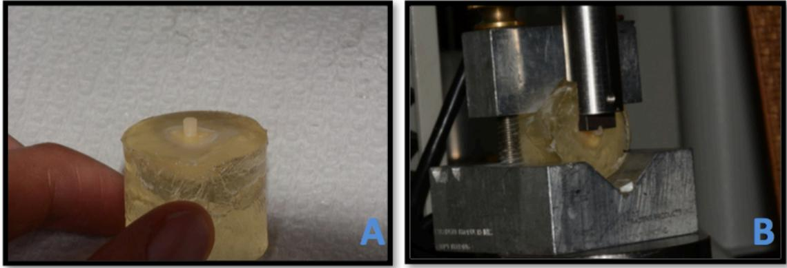
**Figure 5:** A) Specimen for SBS testing B) A specimen mounted in the Instron machine.
