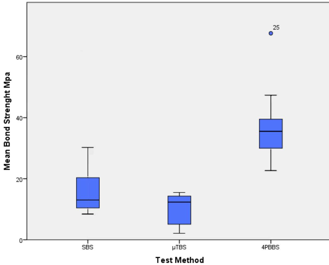
**Figure 9:** Mean Dentin Bond strength of Fuji II LC by test method.
