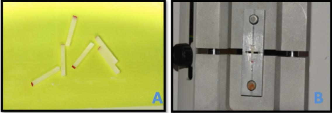
**Figure 6:** A) Beams (~ 1 mm x 1 mm x 6 mm) prepared for  $\mu$ TBS testing B) A beam mounted in EZ-test machine.
