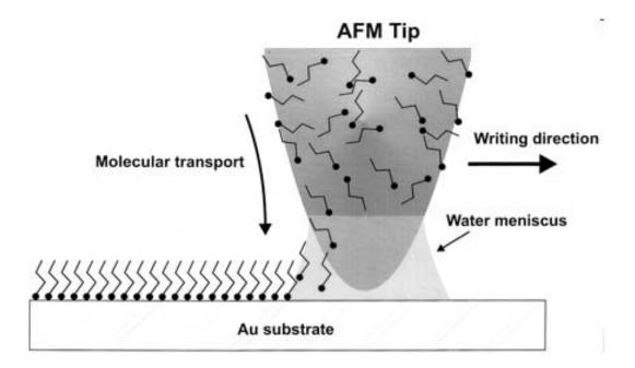
Figure 4-1. Schematic representation of DPN. The figure was taken from reference 1.
