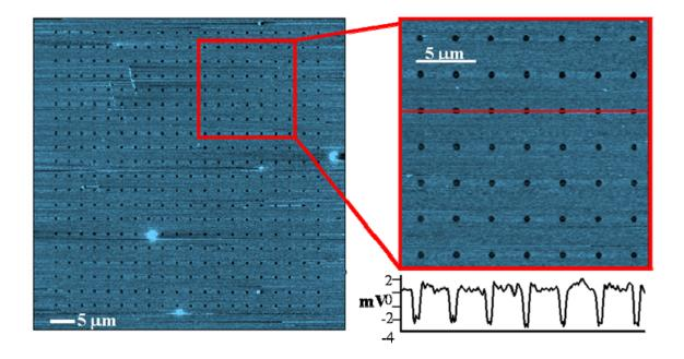
Figure 4-3. Lateral force microscopy (LFM) image of an electroactive nanoarray. The array was generated by DPN of hydroquinone terminated alkanethiol on gold. The array consists of 400 spots ( $20 \times 20$ ) with an average spot size of 500 nm in diameter. Also a lateral force profile for the line drawn across the image is shown.
