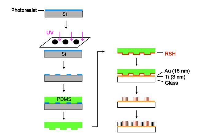
Figure 2-5. Microcontact printing. Microcontact printing is a soft lithography method for patterning SAMs on surfaces. Patterned photoresist serves as a master to generate an elastomeric stamp (PDMS). Alkanethiol-wetted stamp transferred the thiol to the bare gold by physical contact and SAMs are formed in the regions of contact.
