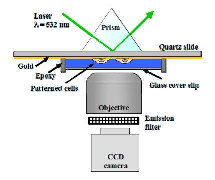
Figure 4-6. Schematic depiction of TIRFM experiment. The sample was placed between a water immersion  $60 \times$  objective and a quartz prism as shown (using water and immersion oil, respectively, for similar refractive indices). Fluorescence excited by TIR was collected through the objective, filtered, and captured on a CCD camera. (Complete optics path has been omitted for clarity.)
