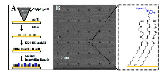
Figure 4-8. Preparation of electroactive nanoarray. A. DPN was used to produce electroactive nanoarrays of hydroquinone-terminated alkanethiol ( $H_2Q-C_{11}$ -SH). Following backfilling with EG<sub>4</sub>-SH, the nanoarrays were electrochemically oxidized and an oxyamine-tethered ligand (linear RGD-ONH<sub>2</sub>) was chemoselectively immobilized. B. Expanded lateral force microscopy image of an electroactive nanoarray on gold.
