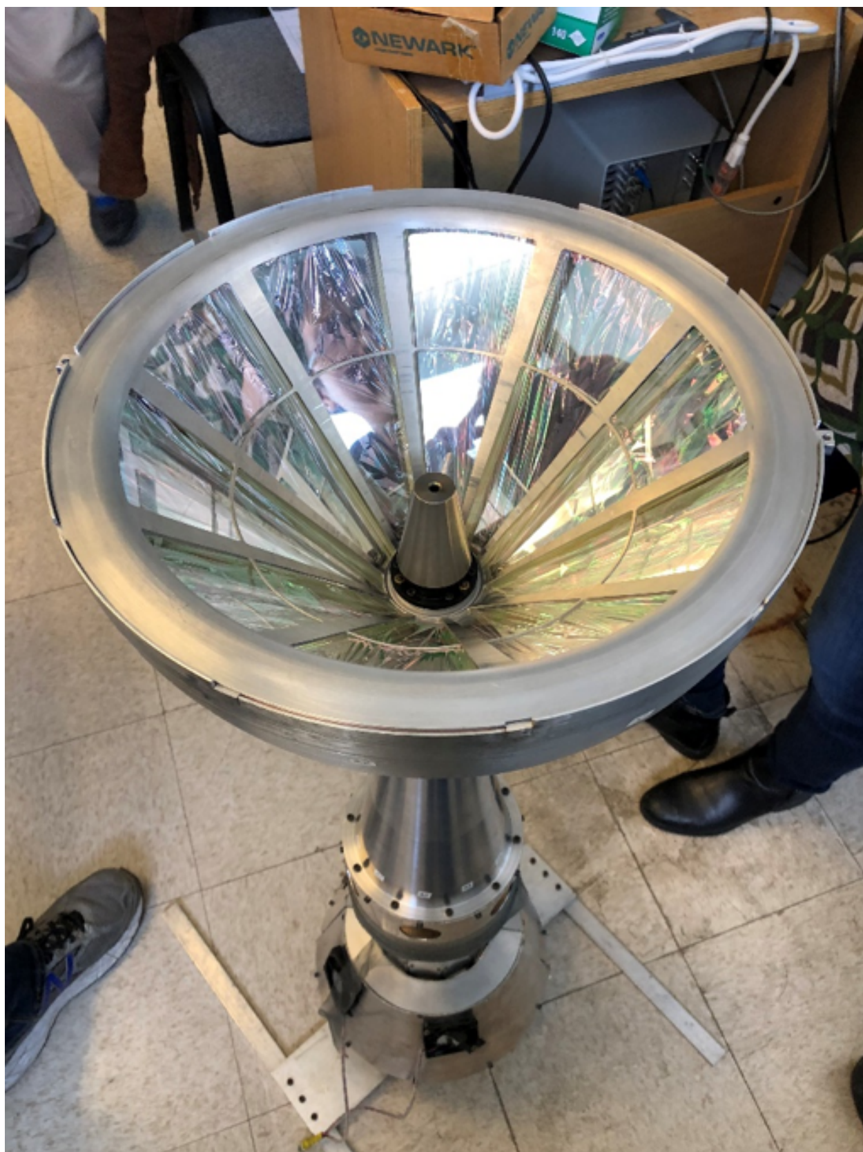
Figure 3.14: Photograph of a single hemisphere of CHICO2 including mylar window and collimator.
