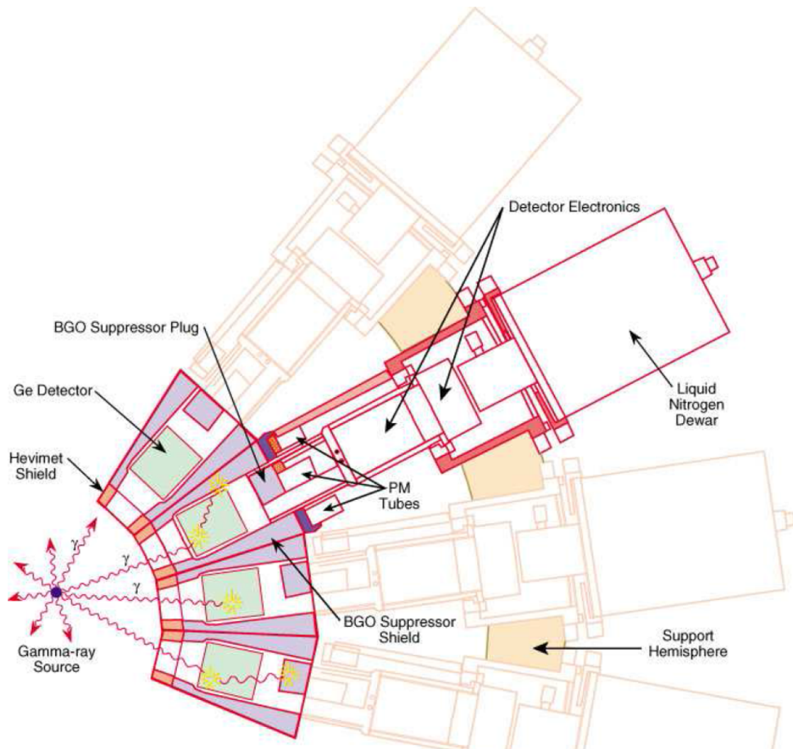
Figure 3.18: Schematic of a Gammasphere detector and cryostat components. The BGO scintillators are in grey, and the HPGe crystals are in green. The orange pieces in front of the BGO detectors represent the heavymet absorbers shielding these scintillators from the \gamma rays emitted at the target.
