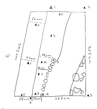
1) 2.865 m = 357.513m2) 2.604 m = 357.513m3) 2.725 m = 357.774m4) 2.955 m = 357.423m5) 3.230 m = 357.423m6) 3.169m = 357.209m7) 3120m = 357.209m7) 3120m = 357.258m8) 3.649m = 356.729m9) 3.725m = 356.653m10) 3.650m = 356.728m11) 3.458m = 356.920m12) 3.454m = 356.920m13) 3.340m = 357.038m14) 3.413m = 356.965m
