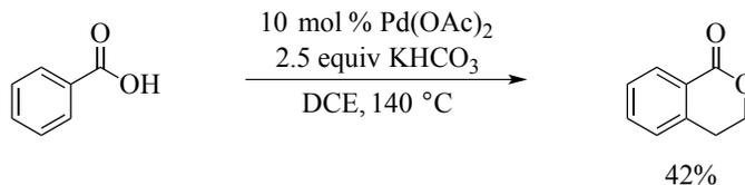
**Scheme 5-4.** Palladium-Catalyzed Ortho Alkylation/Lactonization of Benzoic Acids with 1,2-Dichloroethane
