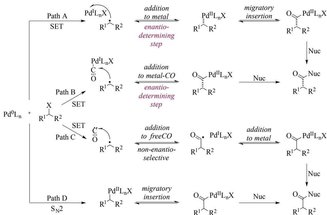
**Figure 4-3.** Potential Mechanisms for the Enantioselective Palladium-Catalyzed Carbonylation
