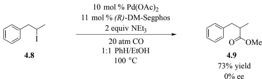
**Scheme 4-7.** Palladium-Catalyzed Carbonylation of Homo-Benzylic Secondary Iodides
