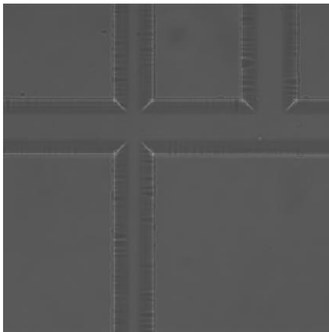
Figure 2.5 Image of a flow through chip coated with APTES/TAMRA demonstrating the lack of cell debris adhesion at the lysis intersection. Approximately 100 cells were lysed with no debris adhesion observed.
