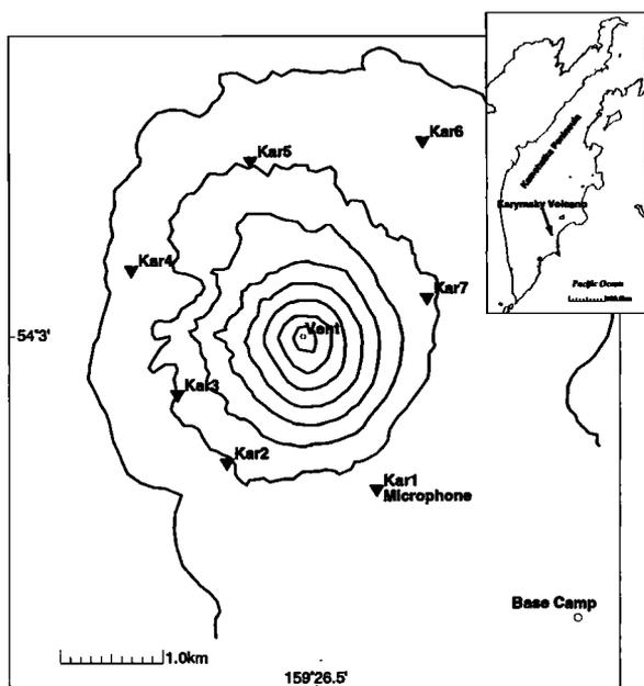
**Figure 1.** Map of Karymsky showing locations of the broadband stations deployed in 1997. Station KAR1 included a broadband microphone as well as a broadband 3-component seismic station. At any given time, only 3 stations were operating. Contours are at 100 m intervals starting at 1000 m. The outer boundary is the rim of a caldera. The inset shows the location of Karymsky on the Kamchatka Peninsula.
