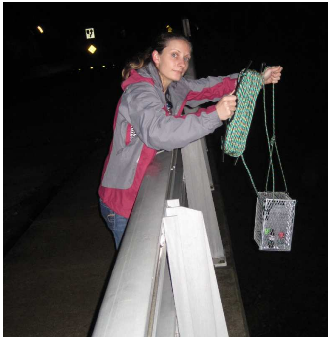
Figure 28: A field technician prepares to collect a sample by lowering the device into the creek below.
