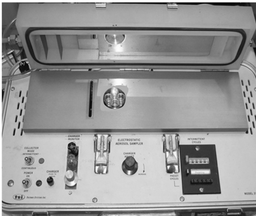
Figure 4: Top view image of the Electrostatic Aerosol In Vitro Exposure System (EAVES) holding the four Millicells
