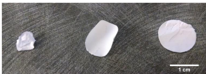
Figure 6.2 Image of electrospun fiber substrates ( 1.267 \text{ cm}^2 ). From left to right: SG 80A/HP 93A, TP 470/SG 80A, and TP 470/HP 93A.
