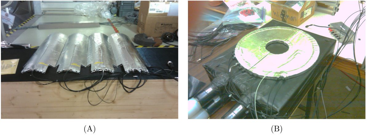
Figure C.4: (A) The long panels layer out side by side. (B) The end caps layer on top of test scintillator panels.
