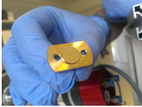
Figure 4.5: The EGun photoelectric surface. This flange is plugged into the backplate to achieve the bias potential. A WLS is inserted in the back to create photoelectrons.
