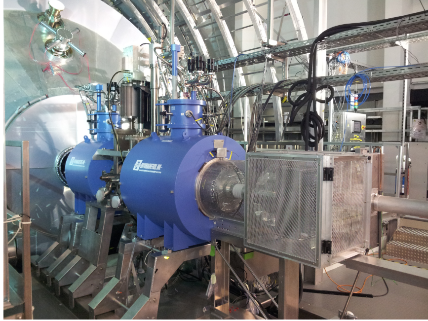
Figure 3.7: The assembled KATRIN FPD system. To the left is the KATRIN main spectrometer. The Faraday cage on the right houses the detector electronics and protects users from the high voltage area of the experiment. Image courtesy of [64]
