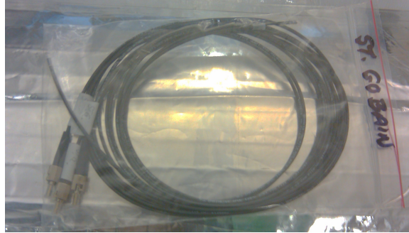
Figure C.2: The St. Gobain fibers used to read out the scintillator panels.
