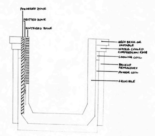
reline by inserting a fabric preliner, grouting cracks around the induction coils and inserting grounding wires, (2) laying the bottom, and (3) building the sides.
