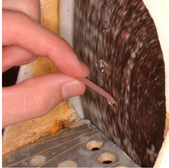
Fig. 12: Preparation of the 45 degree angle in the tray base.
