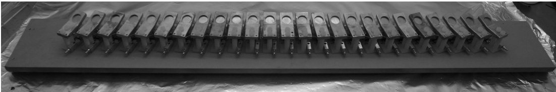
Figure 4-15: Picture of 25 x-ray units on the mounting base.
