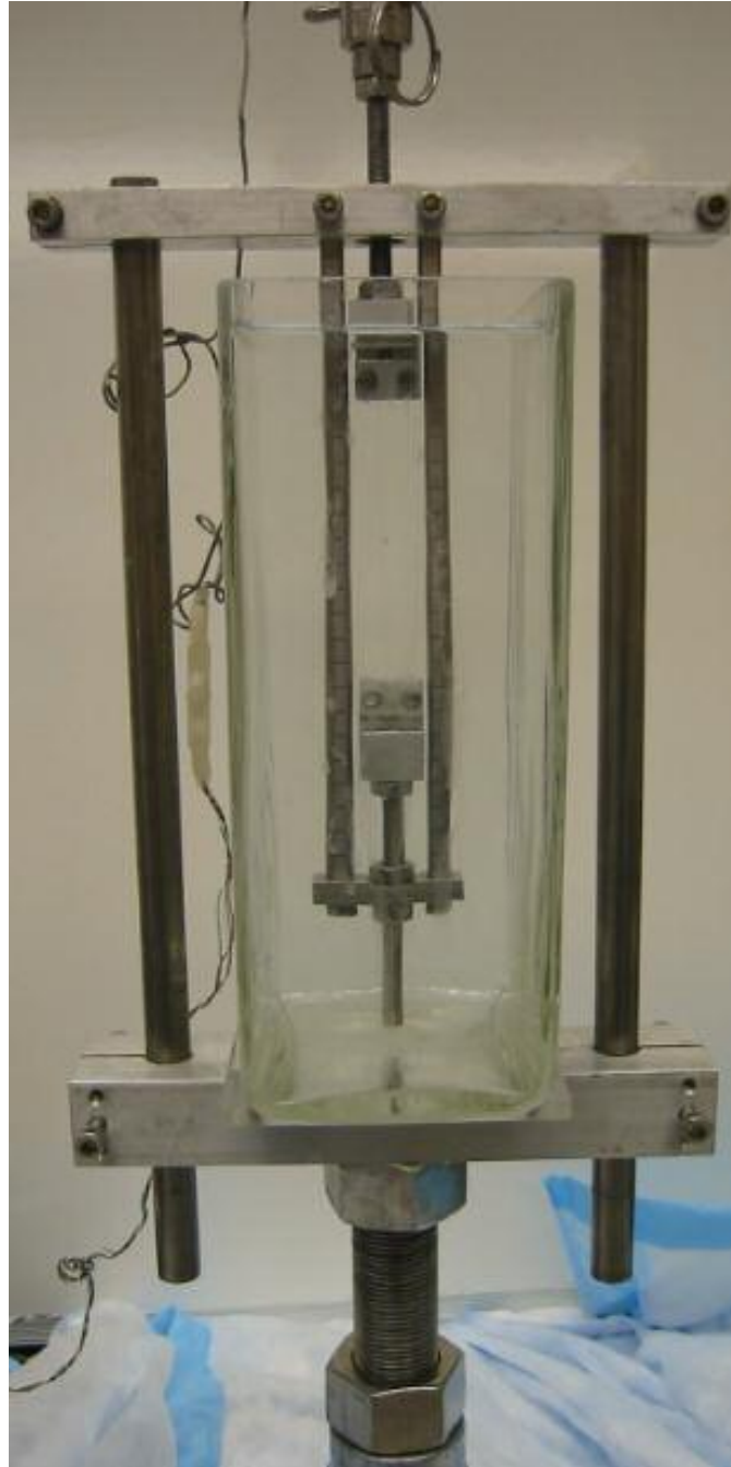
Figure 13: Instron failure testing setup
