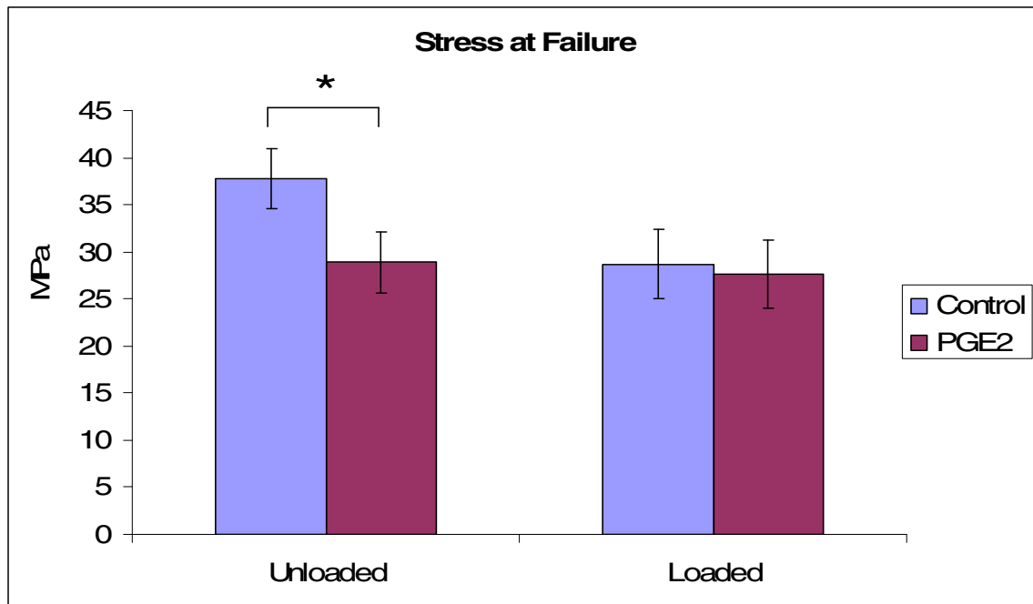
Figure 19: Maximum stress value reached during tensile failure test of rat tail tendon fascicles cultured with and without PGE2 (1 \mu g/ml) and either unloaded for 40 hour culture time, or unloaded for 24 hours followed by 16 hour 0.3 MPa static load in culture. Error bars indicate standard deviation. Asterisks represent significant differences between groups (1-way ANOVA, Tukey's test for multiple comparisons, P < 0.05 ). Sample sizes were as follows: Control (n=15), PGE2 (1 \mu g/ml) (n=10), PGE2 (1 \mu g/ml) plus broad MMP inhibitor (bMMPi, 5 \mu M) (n=12), and PGE2 (1 \mu g/ml) plus specific MMP-3 inhibitor (sMMP3i, 50 \mu M) (n=12).
