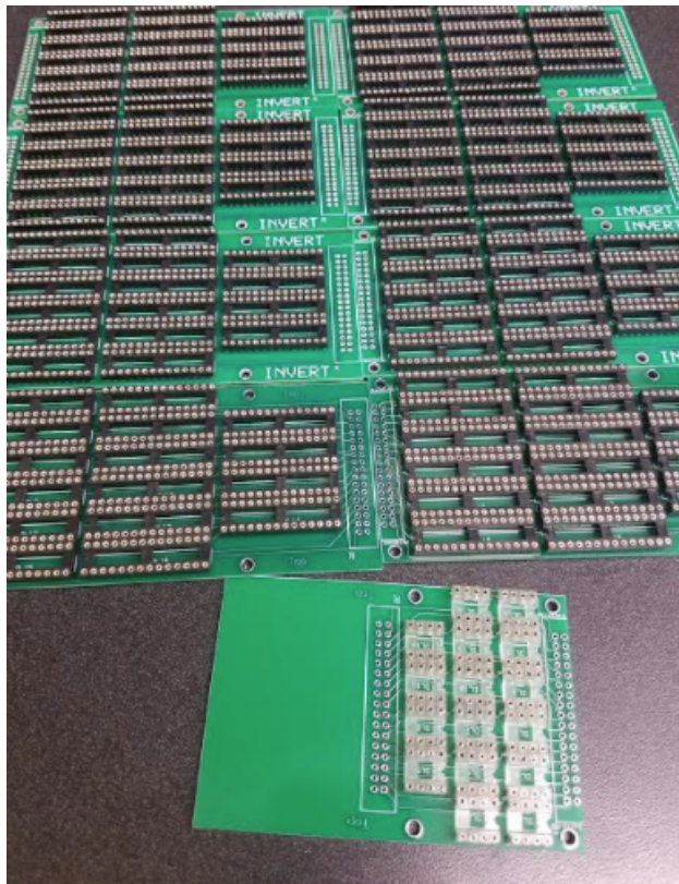
Figure 2.15: IC sockets soldered onto the PC boards, about halfway through the construction process of the delay boards.
