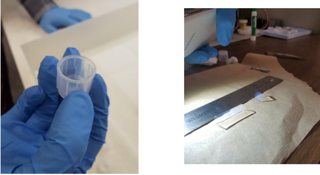
Figure 2.5: Cut aerogel cylinder held in small plastic container (left) and aerogel illuminated by external light (right, faint blue).
