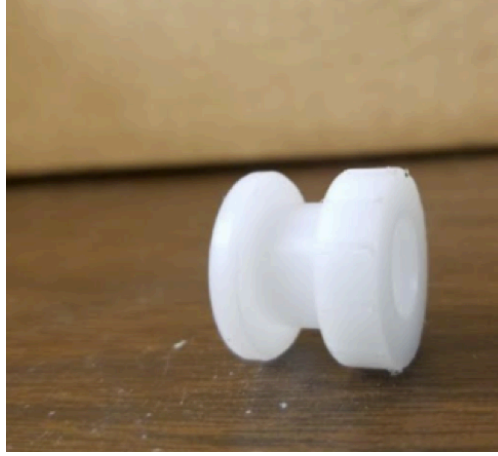
Figure 2.4: Photograph of delrin source holder before insertion into the carbon fiber tube.
