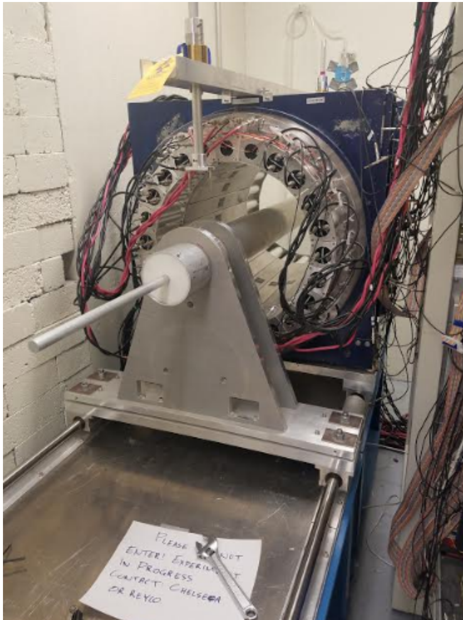
Figure 2.8: The collimator tube inserted inside the APEX array.
