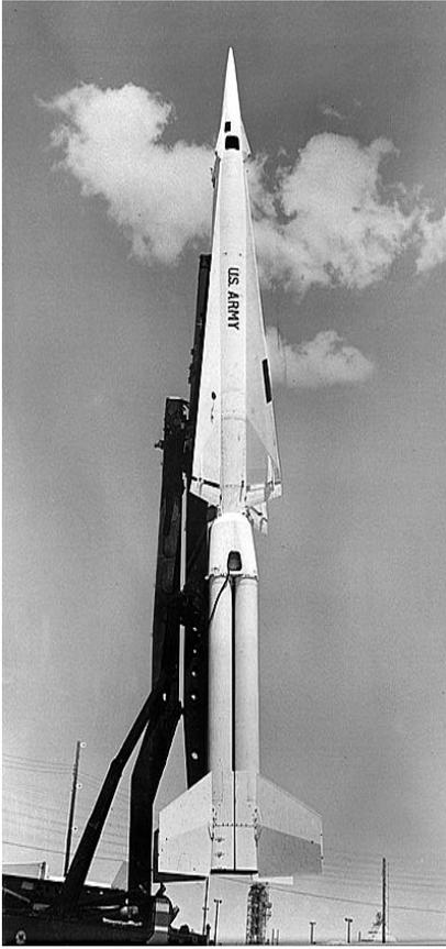
The Spartan interceptor missile was the heart of the Safeguard ABM system
