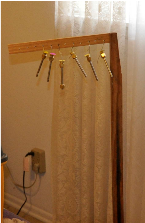
Figure A.1. An example of the passive sampling set up used in residential homes in this study.
