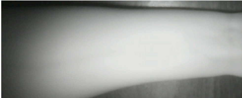
Fig. 12. Sample Colored Image of Forearm Under 910nm exposure. The distance between the subject and camera lens was 20cm and the illumination ring was emitting 910nm light.
