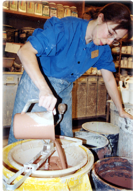
Illustration 19: Sarah Gamble straining glaze through a sieve
